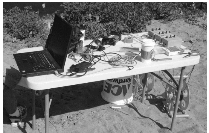
Figure 1. Original hydrophone system made of lab-grade equipment
