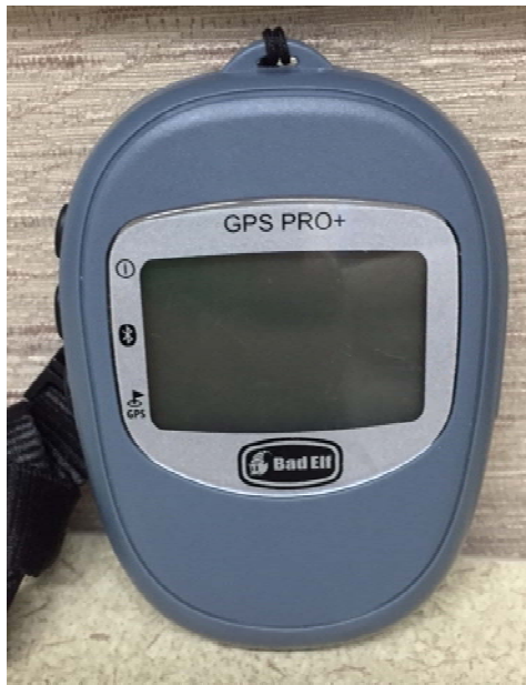
Figure 3. External GPS receiver, the Bad Elf Pro, is attached to a lanyard that you can wear around your neck. The Bad Elf must be within 10m of tablet device for Bluetooth connection to continue working.
