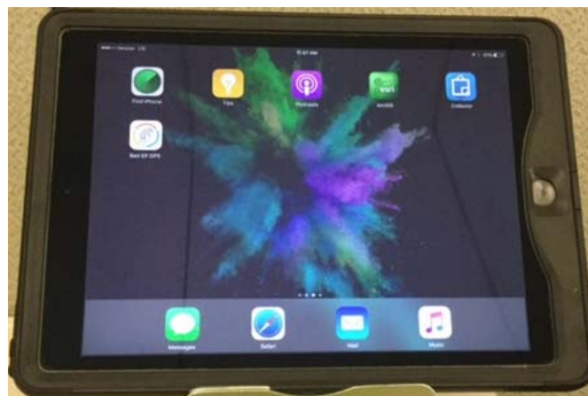
Figure 2. Apple iPad Air 2 device outfitted with a LifeProof Fre case that is water, dirt, snow, and shock resistant. The LifeProof case also has a hand strap attached in the back for easy transport.
