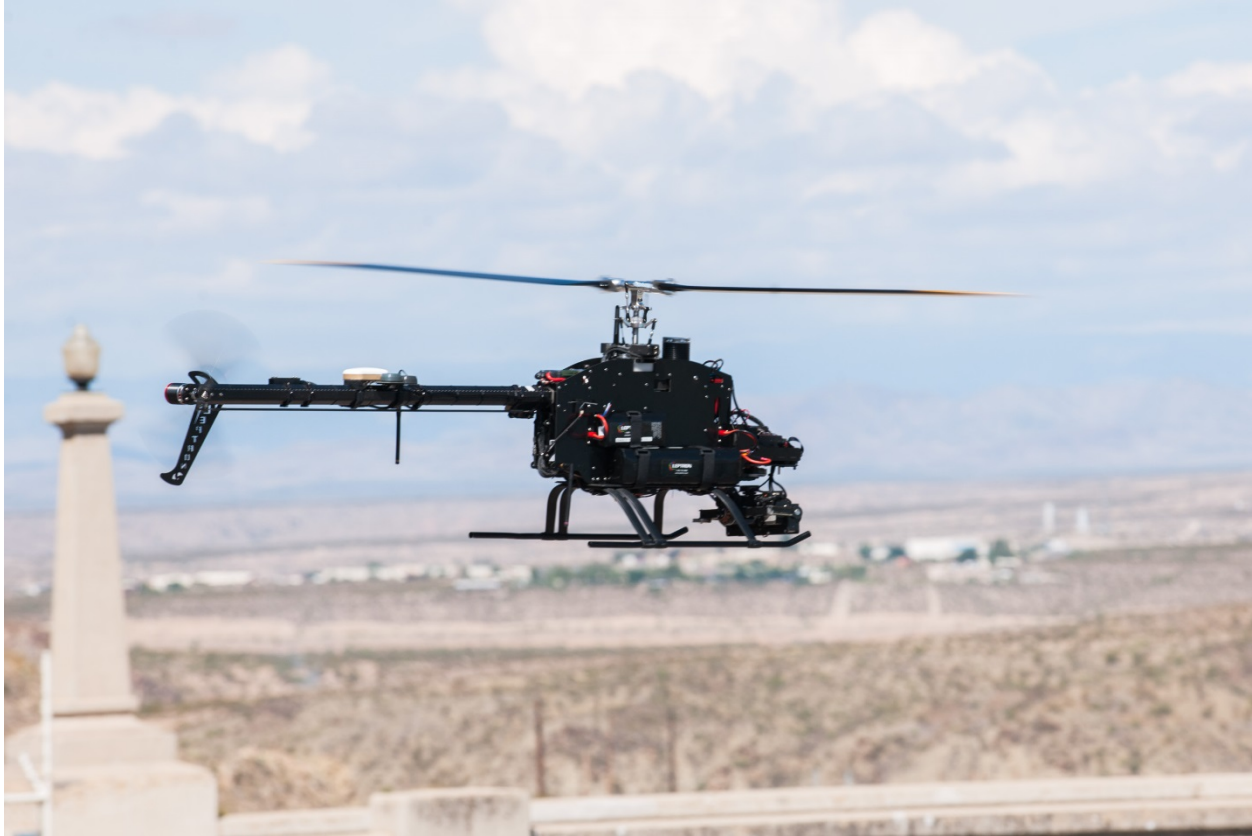
Figure 6: Lepton Avenger E UAS at Elephant Butte Dam (note sensor gimbal at the front of the airframe)
