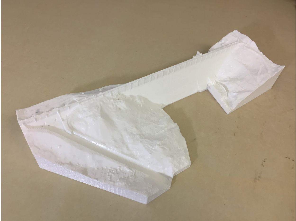
Figure 10: 3D Print of the Photogrammetric Model of Elephant Butte Dam
