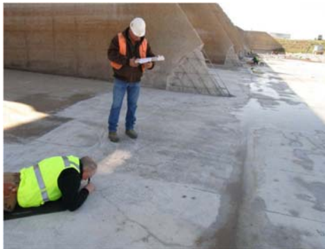
Figure 21. Measuring crack openings.
