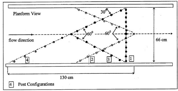
Figure 4: Tested flume post alignments (Wallerstein, Thorne, & Abt, 1997). Alignment 2 (a downstream pointing "V") had the best debris retention with the least backwater.
