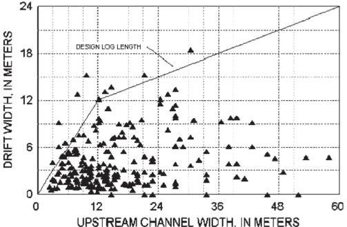
Figure 1: Width of inferred single-pier drift accumulations at scour-potential (e.g. bridge pier) sites in Indiana. A design log length for use in estimating the potential for drift accumulation is inferred from the width of the largest single-pier accumulations and the longest blocked spans; plot source: Diehl, 1997
