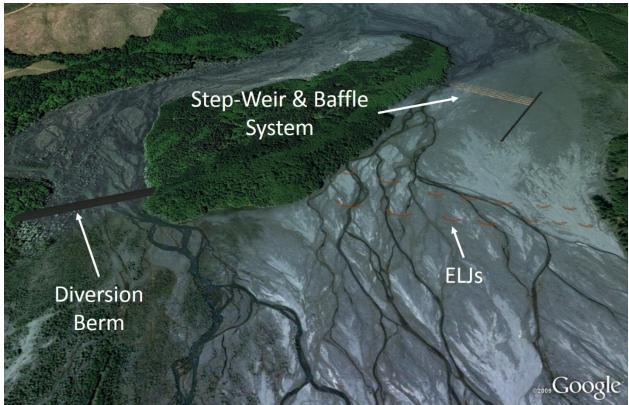
Figure 5: Sediment Retention and Grade Building structures (U.S. Army Corps of Engineers, 2016)
