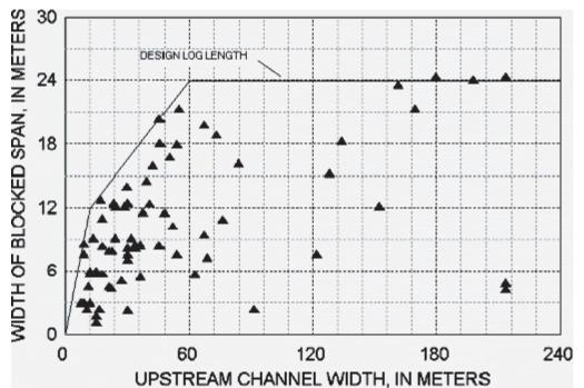
Figure 3: Effective width of drift-blocked spans outside the Pacific Northwest; plot source: Diehl, 1997
