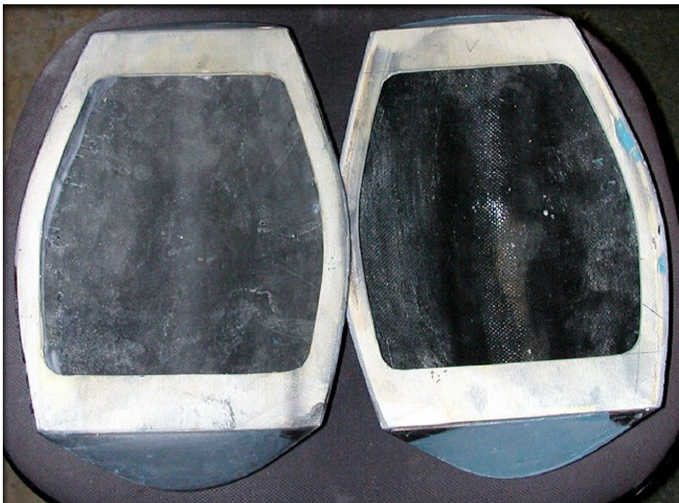
Figure 5. The canopy on the left was vacuum bagged. The canopy on the right was a hand layup. The vacuum bagged version has much less resin on the inside, (less shiny) and it weighs 25 percent less. [15]
