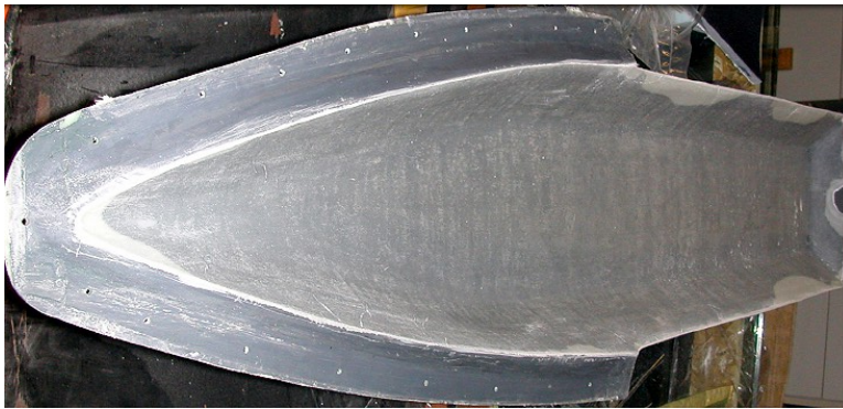
Figure 6. The top photo shows the glass is pulled down firmly into all the corners. The bottom photo shows the finished product which is very dry, light, and neat layup, thanks to the vacuum. [15]
