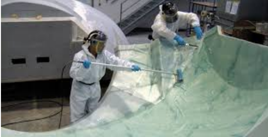
Figure 3. Manual lay-up process for constructing a composite structure. Photo shows a worker applying resin with a roller to the reinforcing fabric. [13]
