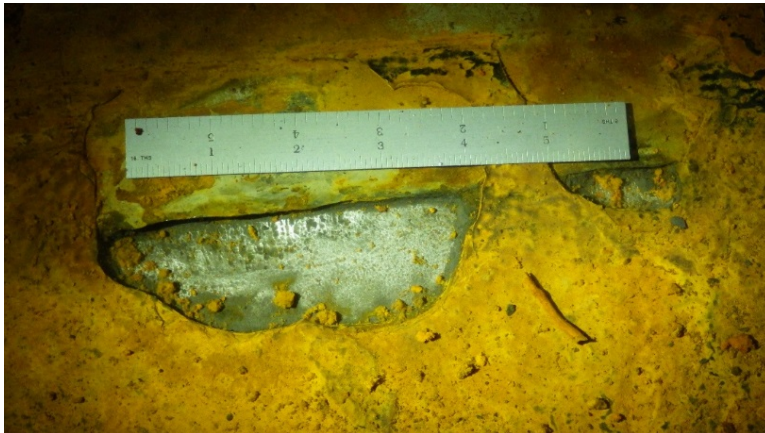
Figure 14. Stainless steel welded to mild steel at Ridges Basin Dam. The uncoated stainless steel gate and gate housing is causing the mild steel to corrode and undercut the weld as well as causing corrosion downstream of this area.
