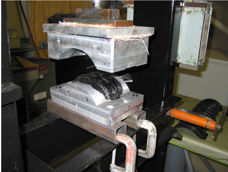
Figure 8. Pre-preg compression molding system showing how a mold or machine is used to form pre-preg fabrics into the final desired shape. These molds are sometimes heated to aid in the curing process. [17]
