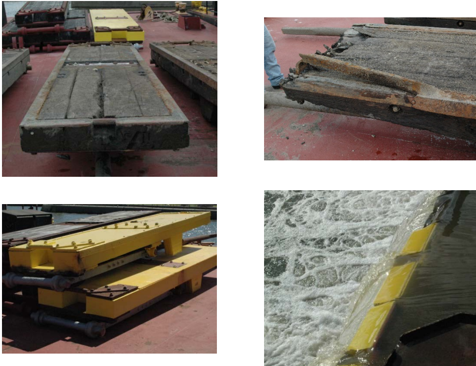
Figure 16. USACE wicket gates at Peoria Lock and Dam. The wooden gate on the left is the wooden constructed style of gate and the gate in the middle is glass fiber reinforced gate being currently field-tested. The image on the right is the installed composite wicket gates being field-tested.
