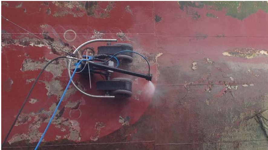
Figure 4: VertiDrive M3 magnetic crawler
