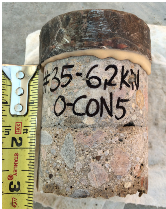
Figure 17. – Example of substrate failure in the pull off test.
