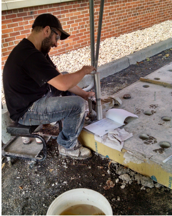
Figure 14. – Pull off testing with the Germann Instruments equipment.
