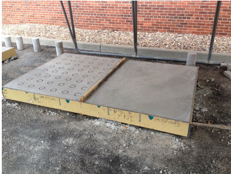
Figure 12. – Marking of the test slab surface for pull off testing.
