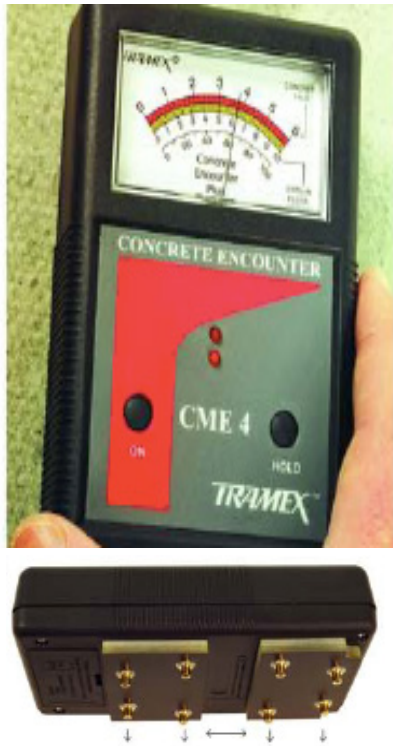
Figure 2. – Devices used to monitor the moisture condition in the surface layer of the concrete specimens: a) electrical impedance surface moisture meter; b) embedded relative humidity probes.
