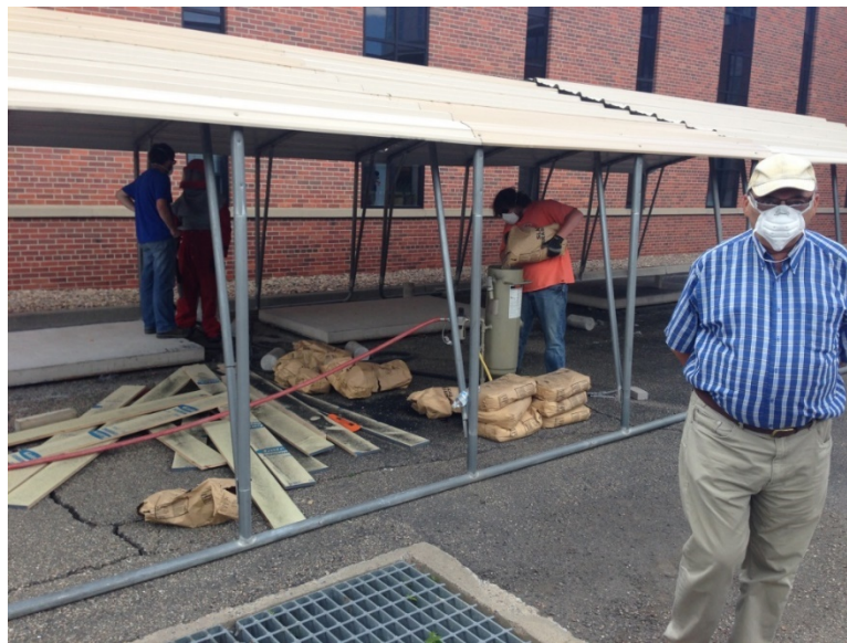
Figure 1. – Surface preparation of the test slabs by sandblasting.
