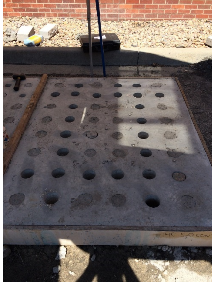
Figure 22. – Long-term pull off testing layout on test slab C2 (MC-5-0-CON7).
