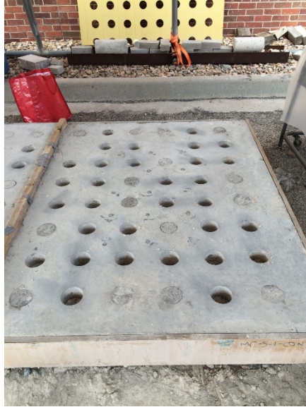
Figure 24. – Long-term pull off testing layout on test slab B2 (MC-5-1-CON7).
