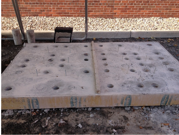
Figure 18. – Short-term pull off testing layout on test slab C (C1: MC-5-0-CON5; C2: MC-5-0-CON7).
