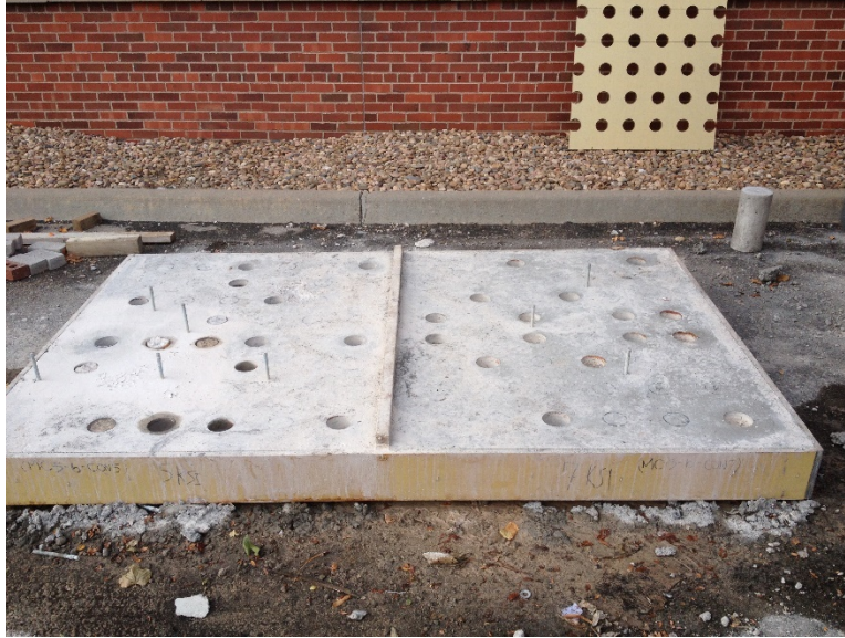
Figure 20. – Short-term pull off testing layout on test slab A (A1: MC-5-6-CON5; A2: MC-5-6-CON7).
