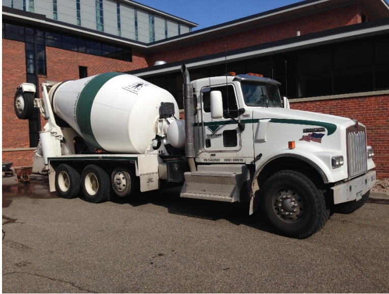
Figure 6. – On-site ready-mix concrete delivery for overlay placement.
