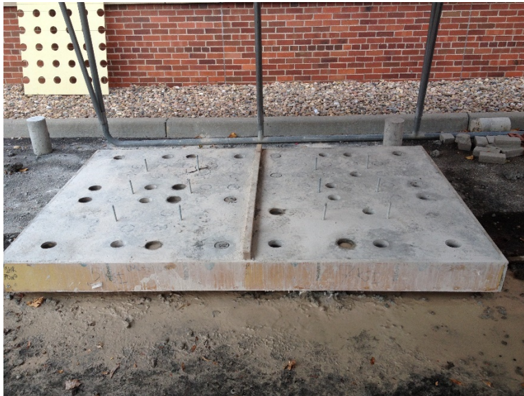
Figure 19. – Short-term pull off testing layout on test slab B (B1: MC-5-1-CON5; B2: MC-5-1-CON7).
