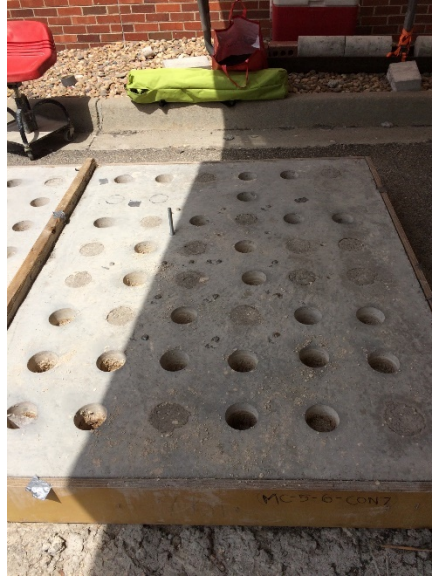
Figure 26. – Long-term pull off testing layout on test slab A2 (MC-5-6-CON7).
