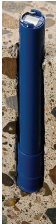
Figure 2. – Devices used to monitor the moisture condition in the surface layer of the concrete specimens: a) electrical impedance surface moisture meter; b) embedded relative humidity probes.
