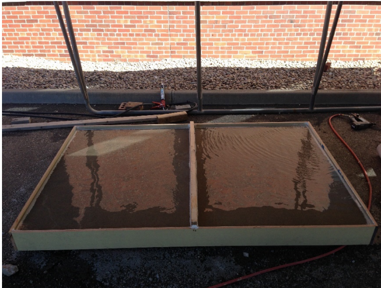
Figure 5. – Moisture conditioning (ponding) implemented on the test slabs prior to overlay placement.
