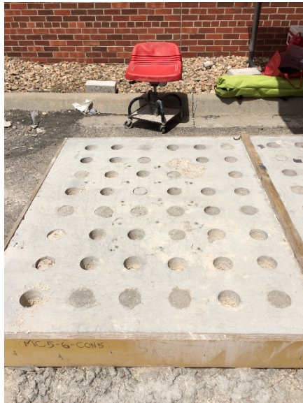
Figure 25. – Long-term pull off testing layout on test slab A1 (MC-5-6-CON5).
