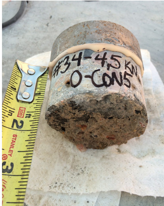
Figure 16. – Example of interfacial failure in the pull off test.
