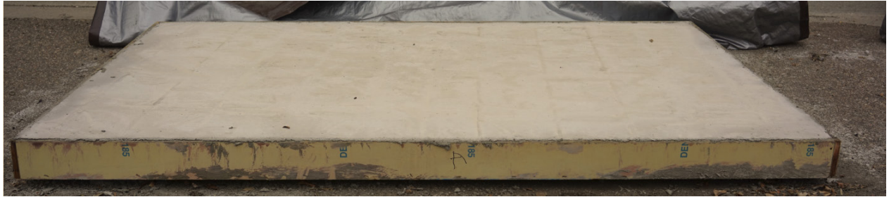
Figure 1. – One of the three 5 by 8 ft cast-in-place test slabs prepared for the field experiments at the Federal Center in December, 2014.
