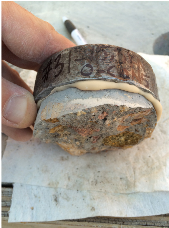
Figure 15. – Example of repair material failure in the pull off test.
