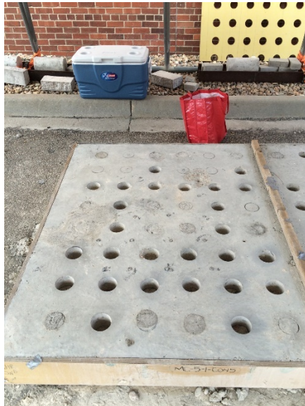
Figure 23. – Long-term pull off testing layout on test slab B1 (MC-5-1-CON5).
