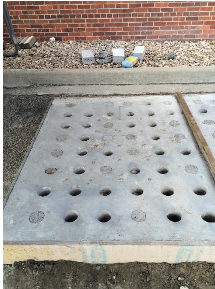
Figure 21. – Long-term pull off testing layout on test slab C1 (MC-5-0-CON5).
