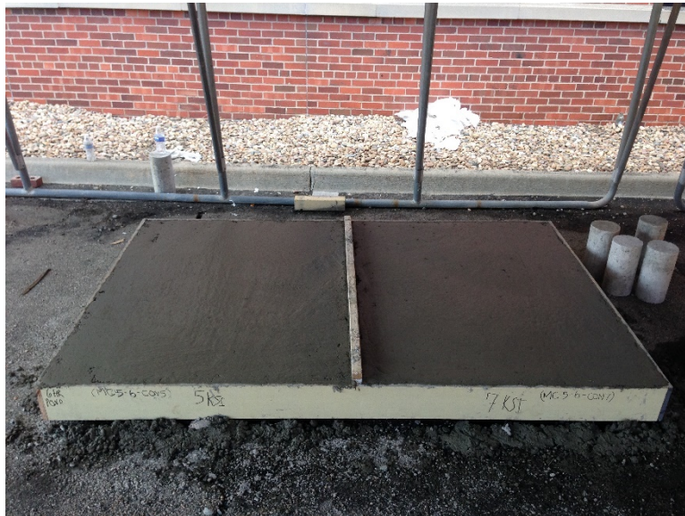
Figure 11. – Overlaid test slab after the finishing operation.
