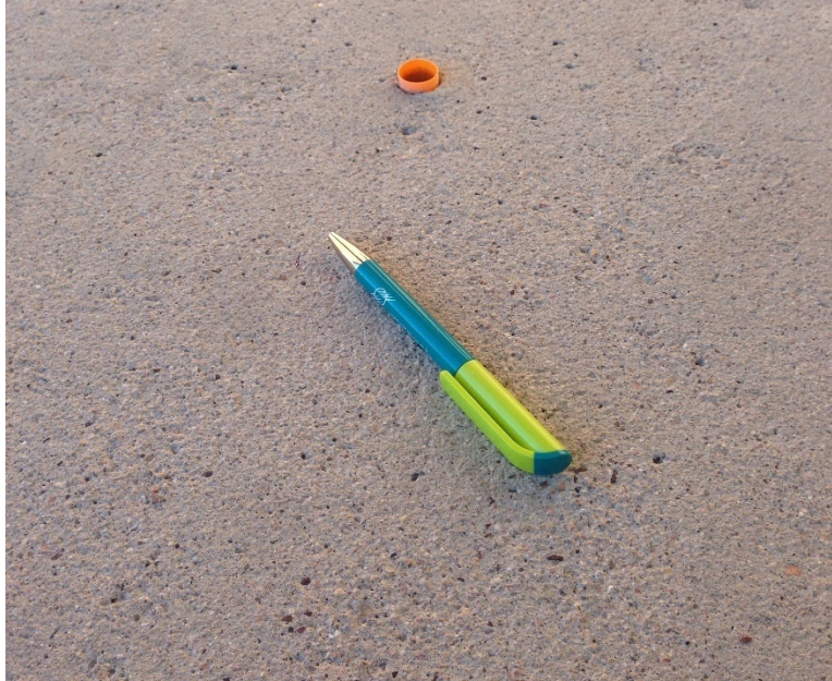
Figure 2. – Surface texture of the test slab after sandblasting and embedded R.H. probe installed for monitoring of moisture inside concrete.
