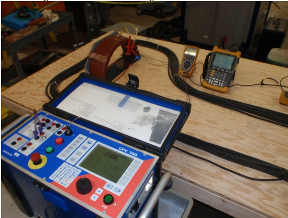
Figure A5- CT excitation test
