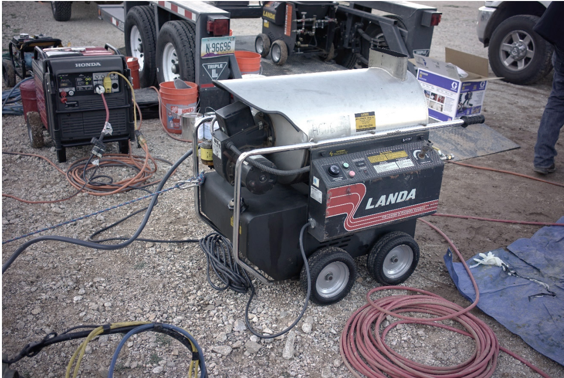
Figure 1 - Water heater and generator for heating premix water
