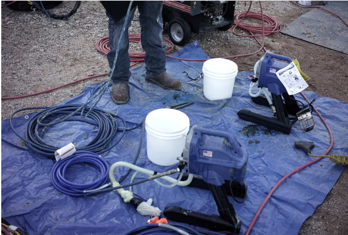
Figure 2 – Airless paint sprayer and hoses for pumping grout and premix water
