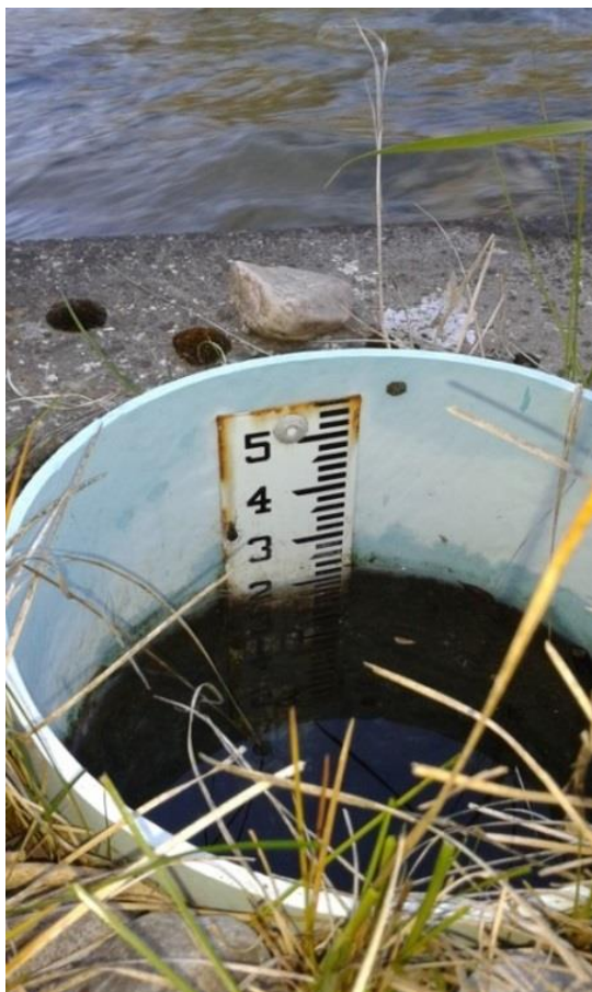
Figure 4.—Upstream six-foot wide Cutthroat flume stilling basin staff gauge for determining flow released from the Upper High Creek Canal headgate. This 1.2 foot staff reading corresponds to 32.1 cfs.
