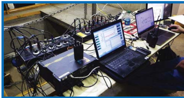
Monitoring for cavitation.
