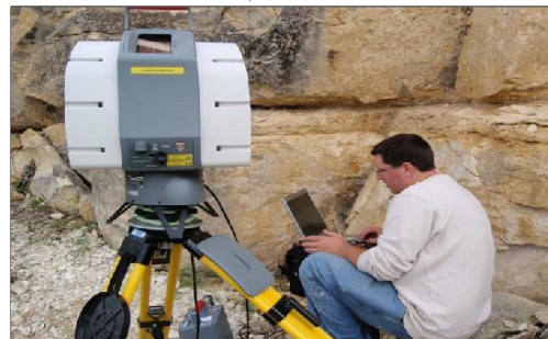
Examining panels using a Leica ScanStation 2.
