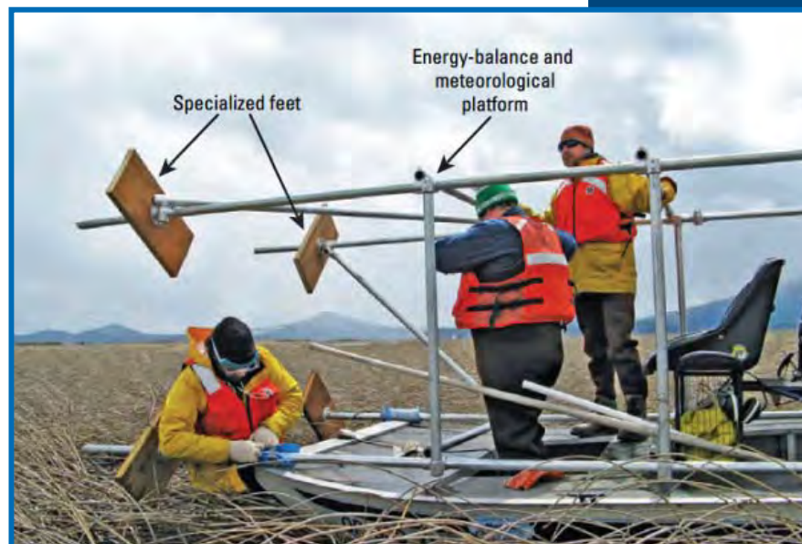
Setting up the ET monitoring equipment for the wetland. Specialized feet support the platform for equipment that measures available energy and meteorological data needed to calculate ET.
