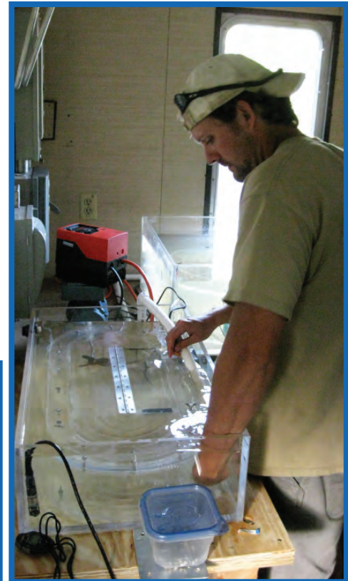
Larval Pacific lamprey being inserted into our fish swimming flume for testing. The fish swimming flume is inside our mobile testing laboratory.
