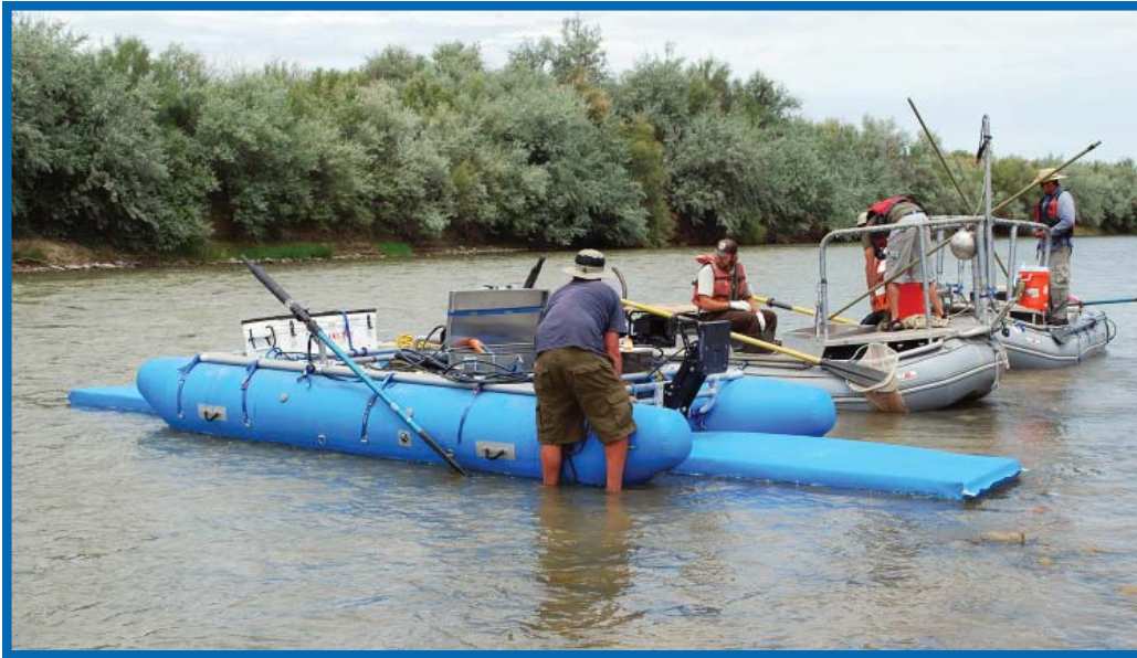
Using PIT tags on floating antenna on the San Juan River, New Mexico.
