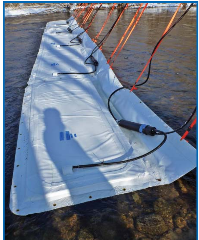
Instream application of new floating antenna system on the Boise River, Idaho.
