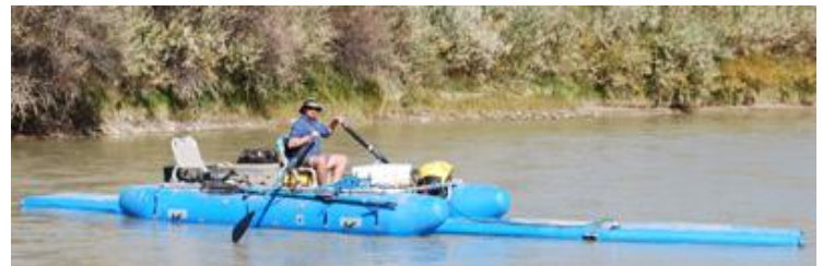
Raft deployed floating PIT tag antennae system on the San Juan River.
