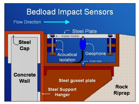
Figure 5. A cross section detail of the weir crest shows the bedload impact sensors and steel gusset support plates attached to the steel cap on the concrete wall.
