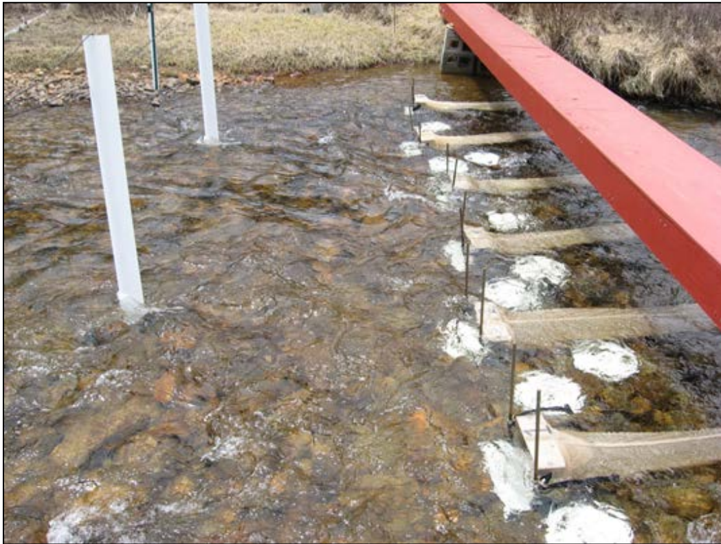
Figure 4: Photograph of the bed load traps deployed at Site 1 in Halfmoon Cr. Flow is from left to right in the photograph. The white posts are the mounting structure for the hydrophones. Photograph courtesy of Dr. Kristin Bunte.
