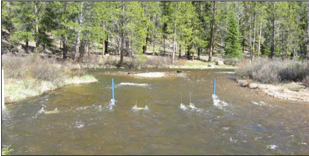
Figure 5: Picture of Site 2 looking upstream. The blue posts are the mounting poles for the hydrophones without the hydrodynamic fairings yet installed. The bed load traps are visible just downstream of the hydrophone mounts. Photograph courtesy of Dr. Kristin Bunte.
