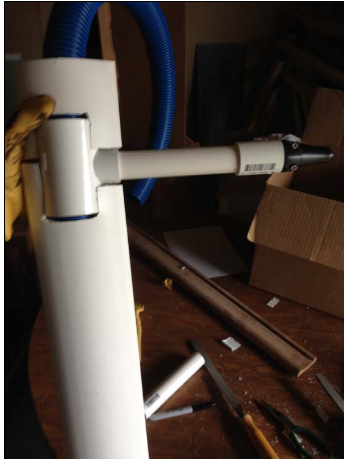
Figure 6: Photograph of the fairing adapted to house the hydrophone. The set-up is upside down in this photo. The hydrophone is mounted inside a black housing 12" downstream of the post and 6" off the
