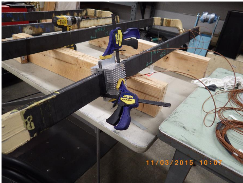
Figure 5: Close-up of Heatsink and Thermocouple Installed on Non-Delaminated Low-Voltage Coil Removed from USBR Generator after 30 Years of Service
