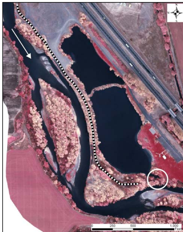
Figure B 2: Aerial photograph showing a floodplain gravel pit with a potential avulsion point at the downstream end shown by the white circle. For the purpose of this discussion, assume that there is a competent levee shown by the dashed line. An avulsion at the downstream end, indicated by the circle, would not create a situation where the river would capture and occupy the gravel pit. This situation poses a lesser risk than if the levee avulsed at the upstream end.
