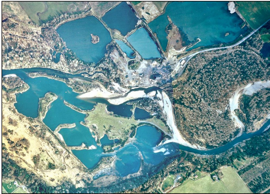
Figure B 1: Aerial photograph showing a bend in the channel alignment (prior to avulsion the channel flowed between the groups of mining pits) forced by the presence of the mining pits. Photograph is of the Daybreak Mine Area on the East Fork of the Lewis River, Oregon ( Photo courtesy of Thomas Grindeland, WEST Consultants).
