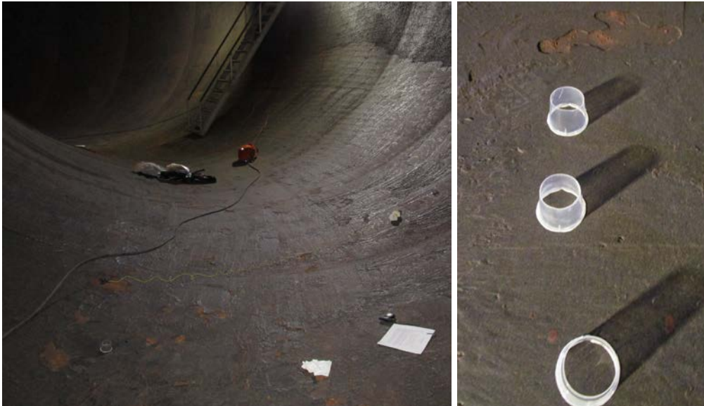
Figure 10. EIS field demonstration at Grand Coulee Dam, Cells 1 and 2 located near the scroll case mandoor (left) and triplicate Cells 3, 4, and 5 (right).
