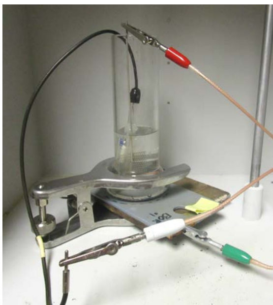
Figure 2. EIS testing three-electrode cell set-up; the colored leads are the working (green), reference (white), and counter (red) electrodes.
