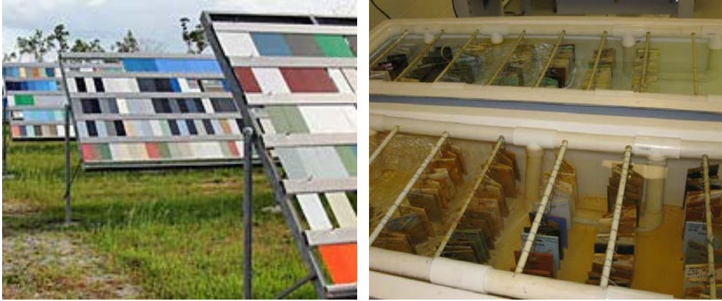
Figure 1. Example weather methods: (left) USACE Paint Technology Center atmospheric test rack and (right) Reclamation immersion tanks.
