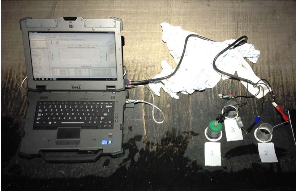
Figure 13. EIS test set-up for two-electrode experiment. Three test cells shown; Cell 1 is reference cell and Cell 2 is working cell in this example.
