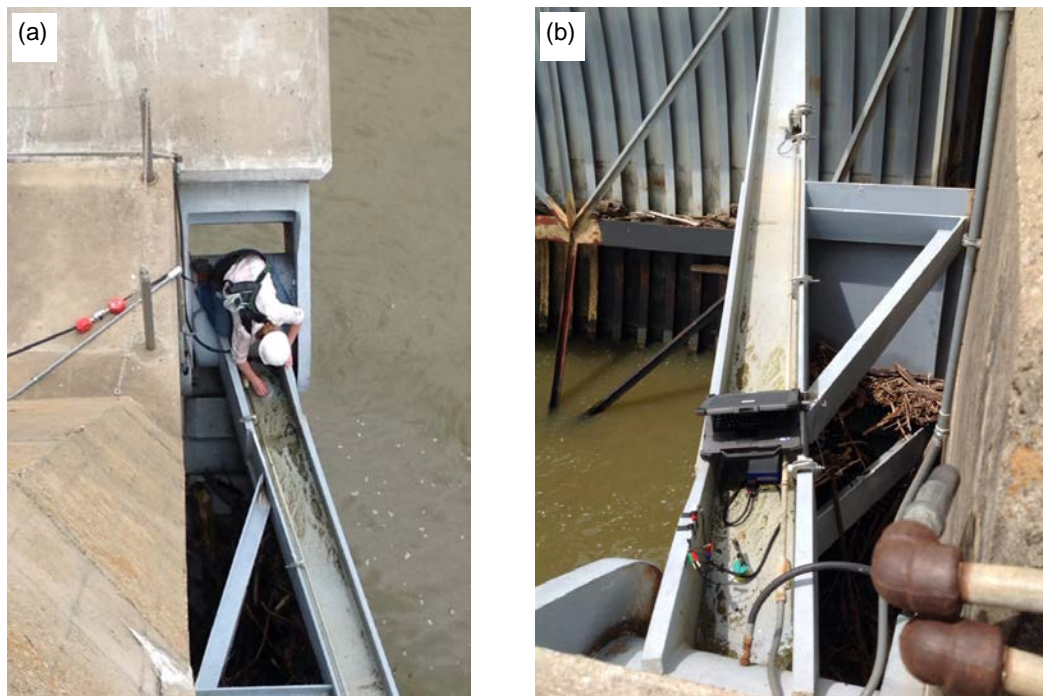
Figure 8. EIS field demonstration at US Army Corps of Engineers' Ozark-Jeta Taylor Lock and Dam (a) test cell set-up and (b) test in progress.
