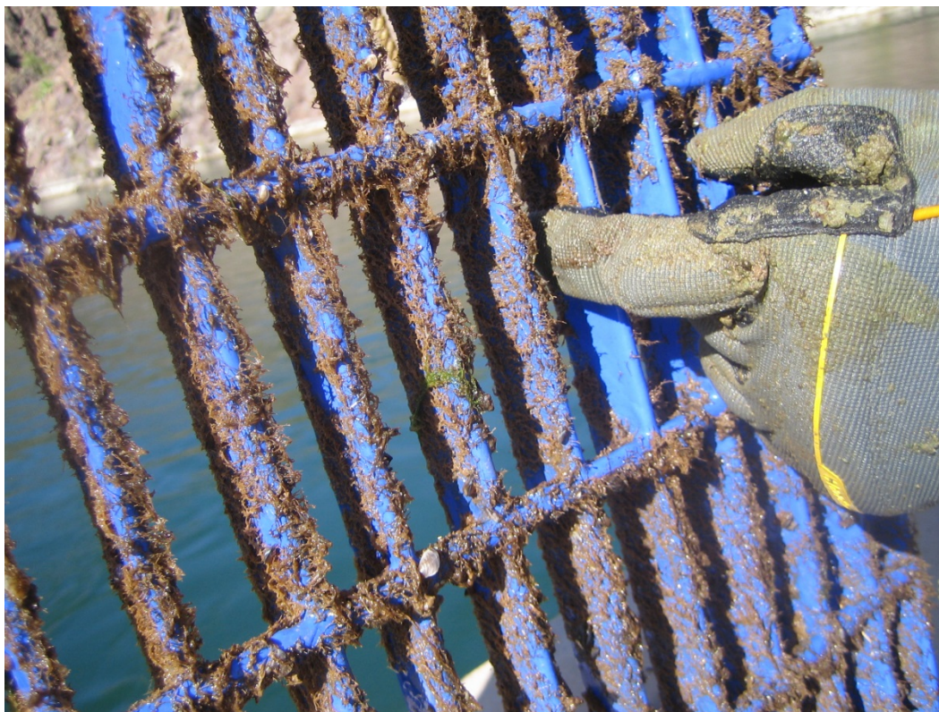
Figure 9.—International Paint Intersleek 970 easily cleaned, inspection date October 2009 after 18 months exposure.
