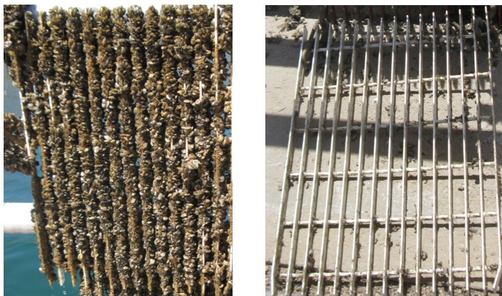
Figure 16.—Grate treated with Nusil R1082 silicone ice phobic coating, before cleaning (left) and after cleaning (right), 12 months.
