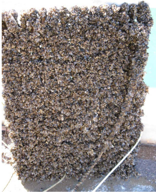
Figure 8.—Uncoated steel after 7 months of exposure in dynamic conditions. Test period May 2008 to December 2008.
