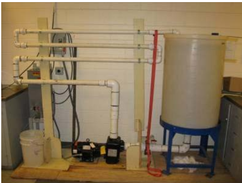
Figure 21.—High flow water test set up. Samples are placed inside 1.5 in PVC pipe.
