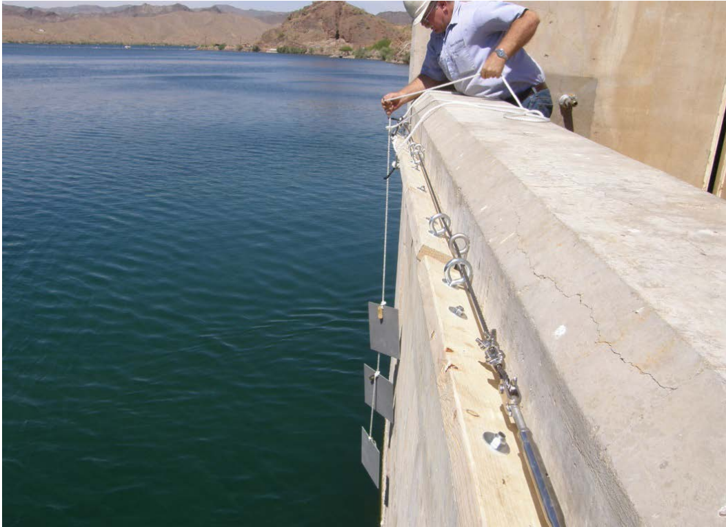
Figure 2.—Coated steel plates placed in static exposure on the face of Parker Dam.
