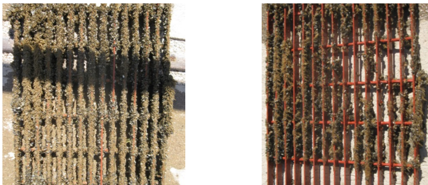
Figure 12.—Jotun Sealion Resilient, as seen in May 2015 (2 years of exposure) before cleaning (left) and, after cleaning by a forceful dip into the water (right).
