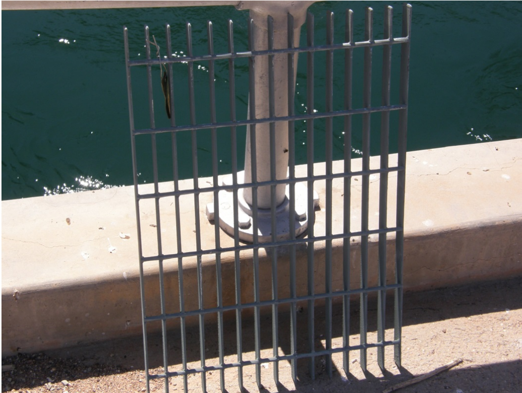
Figure 3.—Coated floor grate before being suspended from the forebay trashrack structure at Parker Dam.
