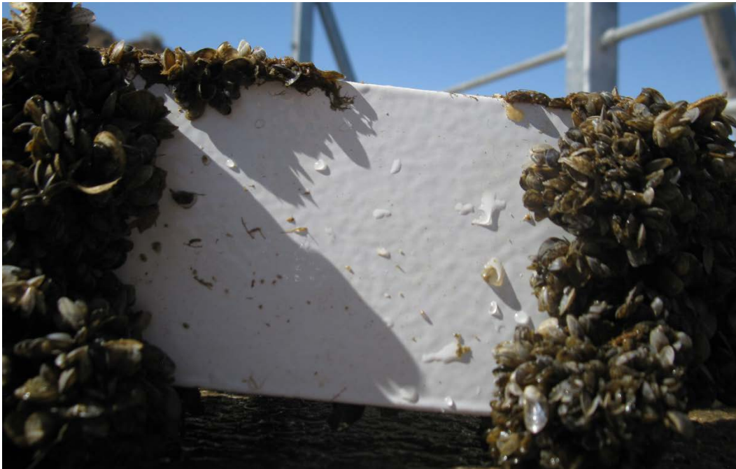
Figure 10.—Fuji Film silicone oil-free after 34 months of exposure.
