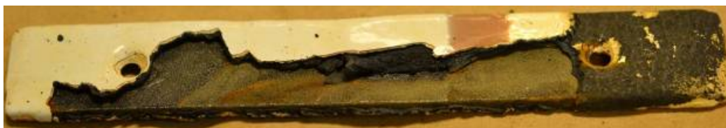
Figure 22.—Failure of overcoated coal tar during a high flow test.
