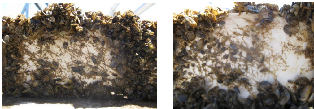
Figure 14.—Panels coated with experimental formulations from 2012-MTA-8-1003 #1 (left) and #2 (right), exposure at 30 months.
