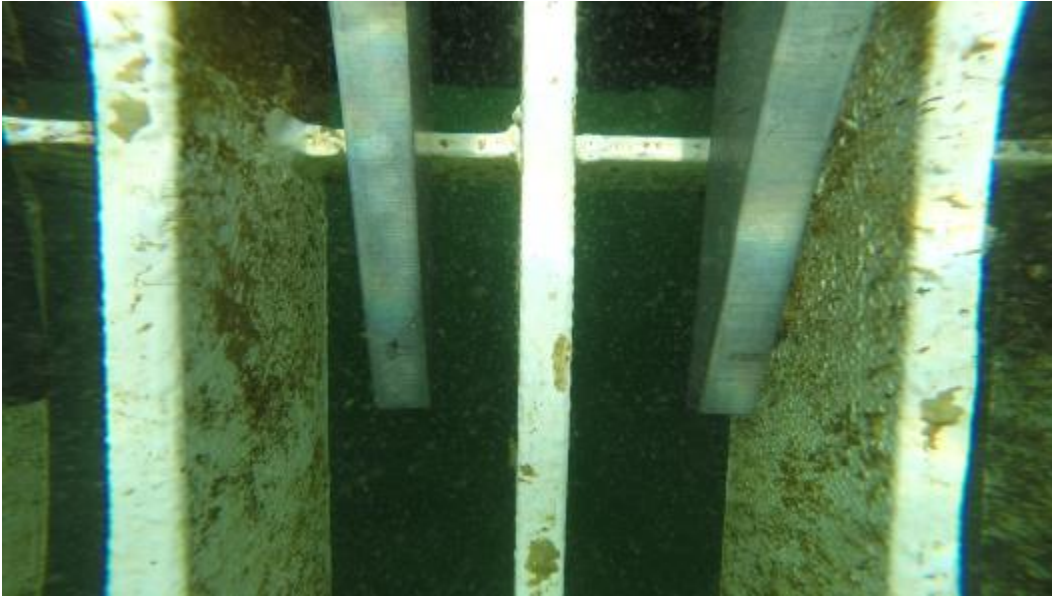
Figure 16.—International Paint Intersleek 970 after 18 months exposure.
