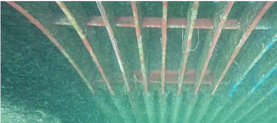
Figure 17.—PPG Sigmaglide 890 after 18 months exposure.
