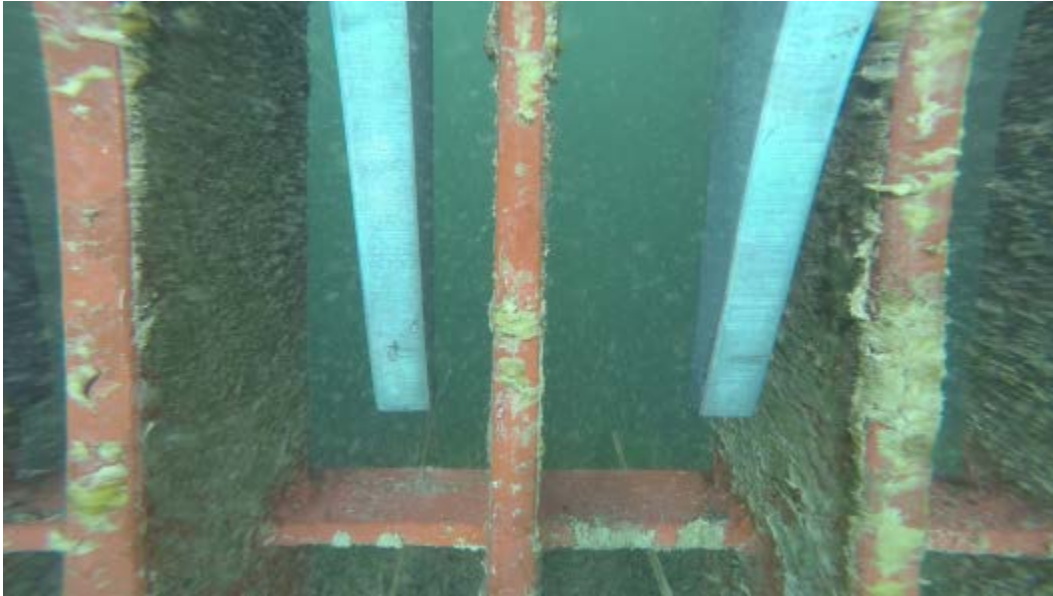
Figure 18.—PPG Sigmaglide 890 after 18 months exposure.
