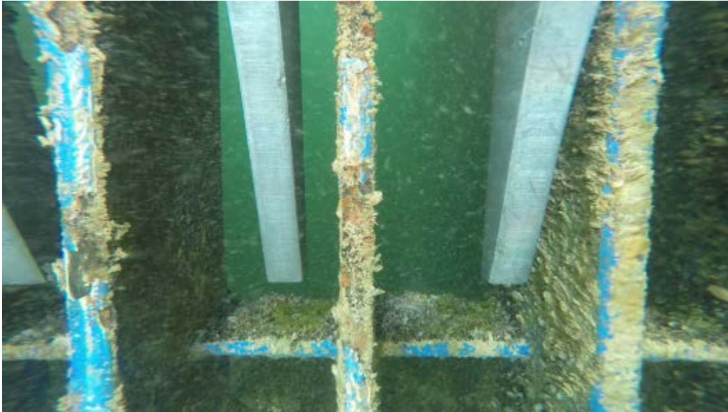
Figure 22.—Seacoat Seaspeed V5 after 18 months exposure.
