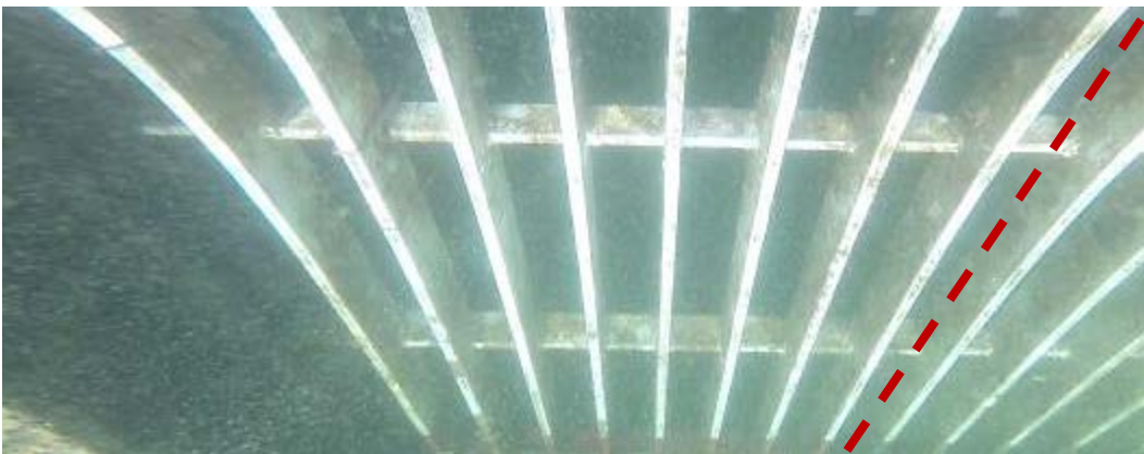
Figure 15.—International Paint Intersleek 970 after 18 months exposure—the dashed line demarcates the end of the Intersleek coating.
