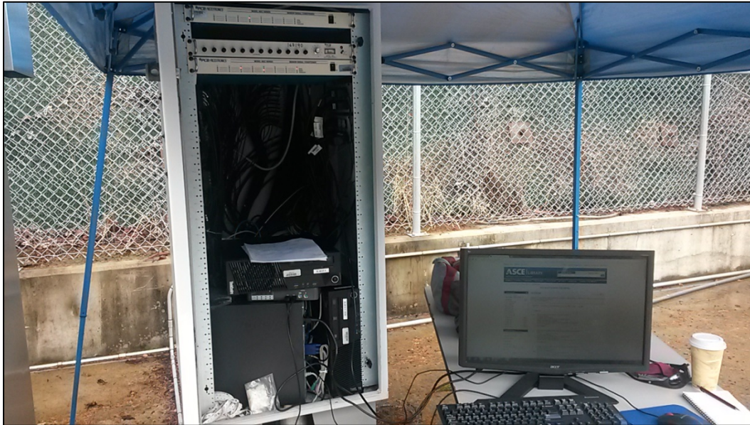
Figure 1: Photograph of the computer cabinet housing the Elwha impact plate system computers. In 2015 a fourth computer was installed and a bad computer was replaced.
