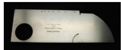
Current reference standards have machined artifacts
