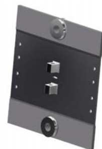
Concept for High-Rate Modified Middle Crack Tension Tests
