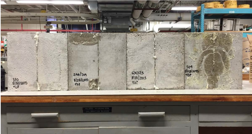
Figure 8. Top view of concrete specimens after underwater grout injection
