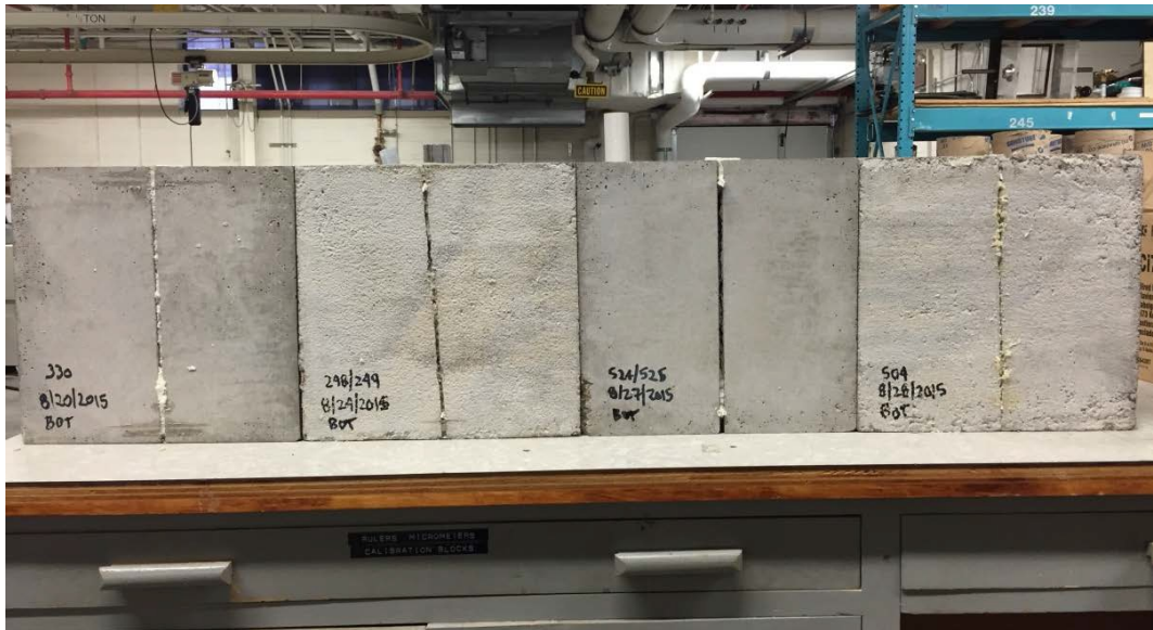
Figure 7. Bottom view of concrete specimens after underwater grout injection
