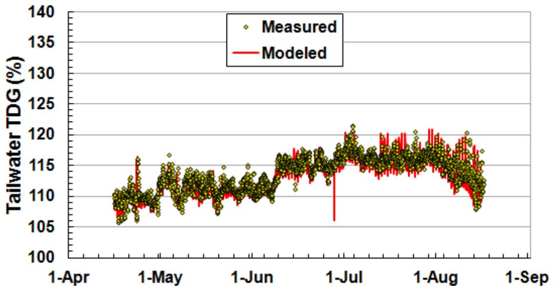
Figure 14: Modeled and measured TDG concentration at Rock Island Dam in 2009
