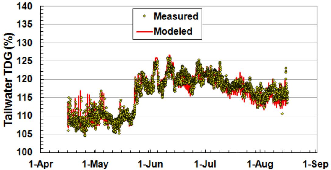
Figure 13: Modeled and measured TDG concentration at Rock Island Dam in 2008
