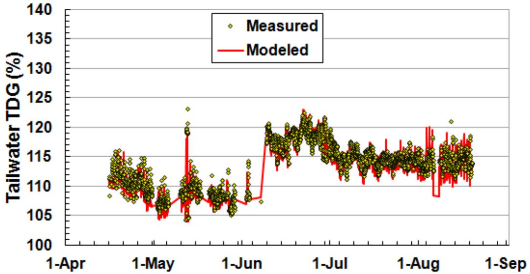
Figure 15: Modeled and measured TDG concentration at Rock Island Dam in 2010
