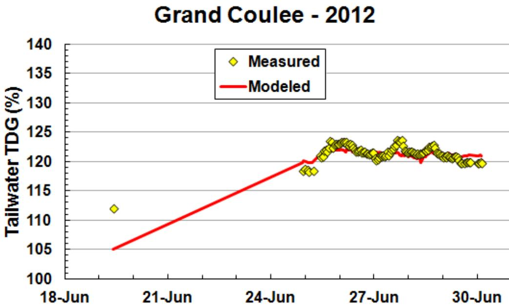
Figure 22: Modeled and measured TDG concentration at Grand Coulee Dam in 2012
