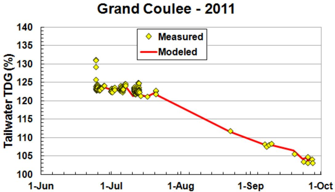
Figure 21: Modeled and measured TDG concentration at Grand Coulee Dam in 2011
