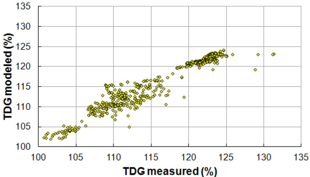
**Figure 23: Measured vs. predicted TDG in the tailrace**
