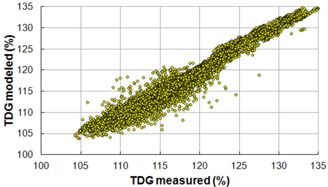
**Figure 18: Measured vs. predicted TDG in the tailrace**
