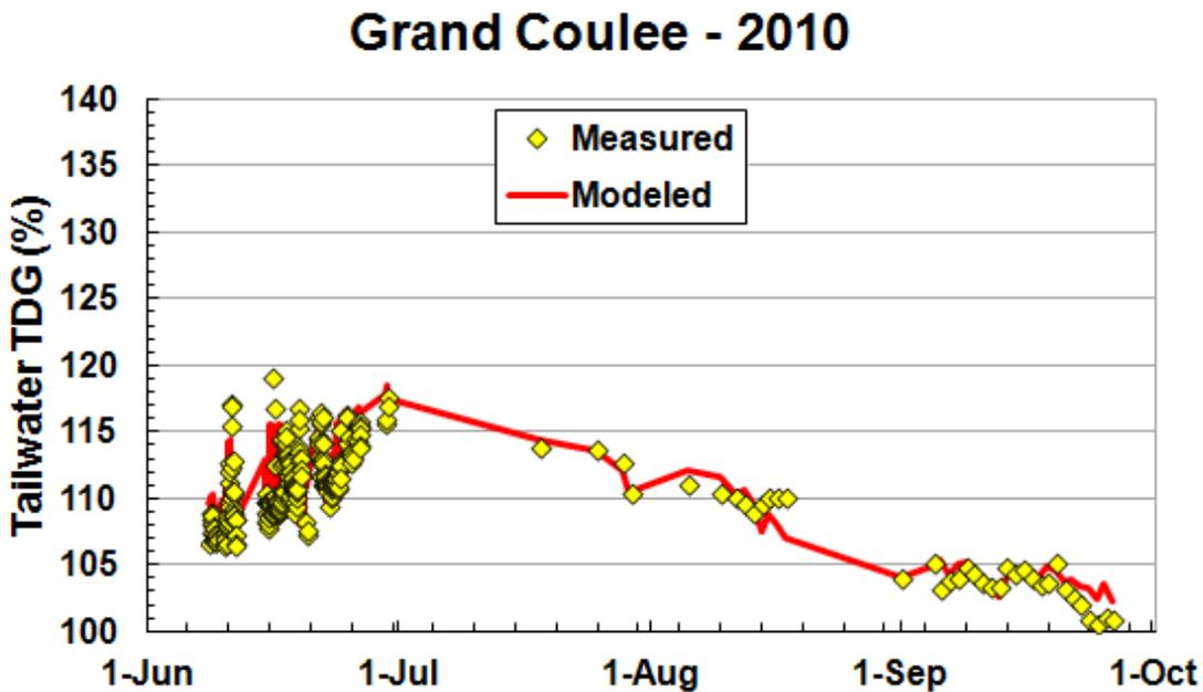
Figure 20: Modeled and measured TDG concentration at Grand Coulee Dam in 2010
