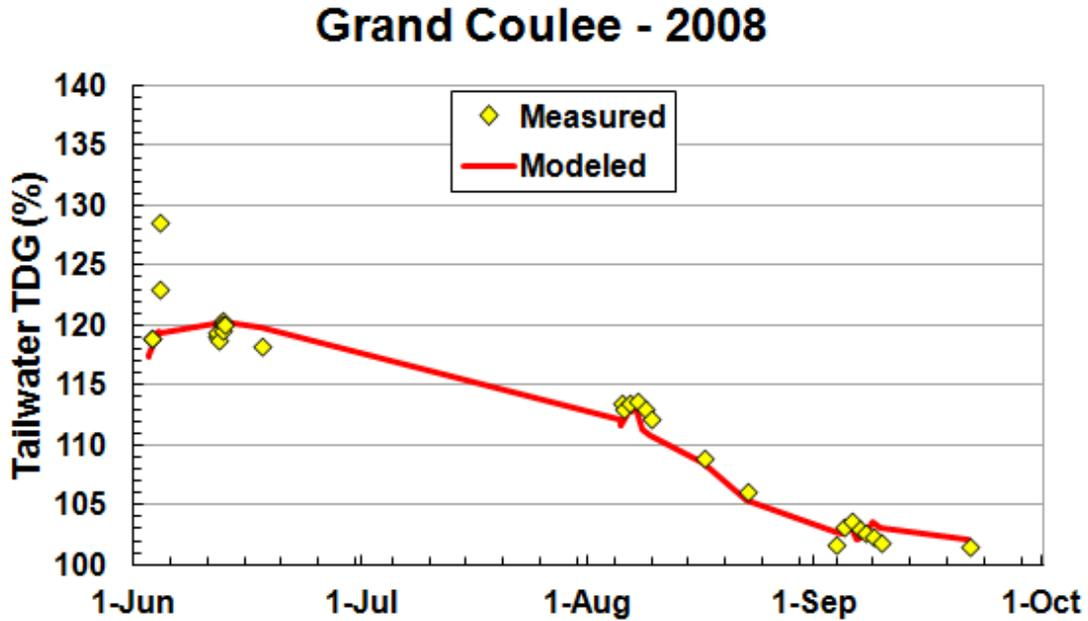
Figure 19: Modeled and measured TDG concentration at Grand Coulee Dam in 2008
