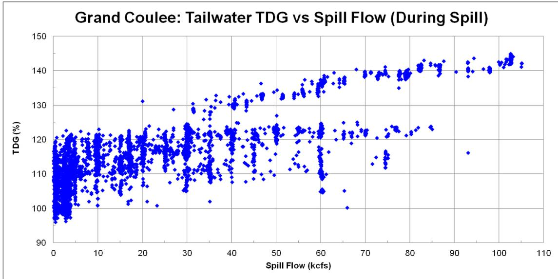
**FIGURE 12: GRAND COULEE TAILWATER VS SPILL FLOW DURING PERIODS OF SPILL**
