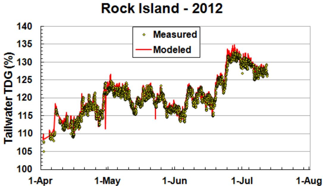
**Figure 17: Modeled and measured TDG concentration at Rock Island Dam in 2012**
