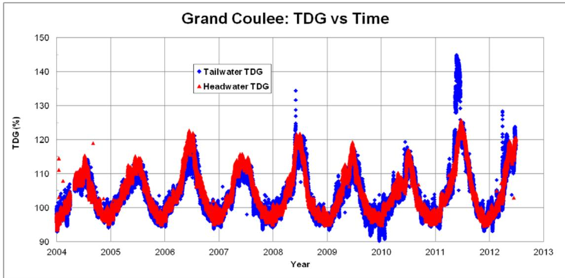
**Figure 10: Grand Coulee forebay (FDRW) and tailwater (GCGW) TDG from 2004 to 2012**
