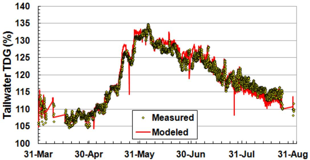
Figure 16: Modeled and measured TDG concentration at Rock Island Dam in 2011
