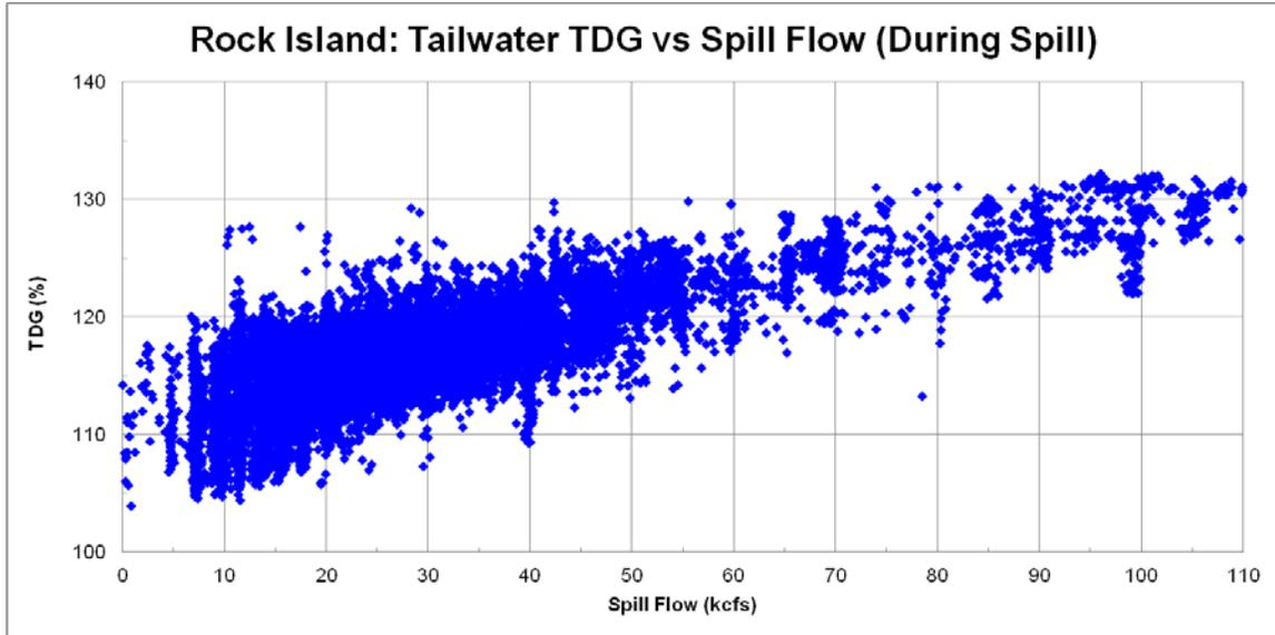
**Figure 9: Rock Island tailwater vs spill flow during periods of spill**
