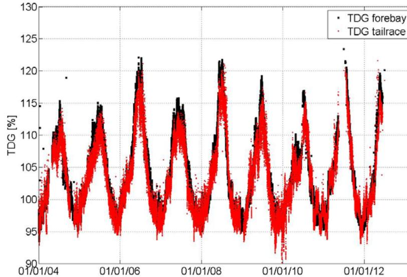
**Figure 11: TDG measured in the forebay and tailrace of Grand Coulee without spill**
