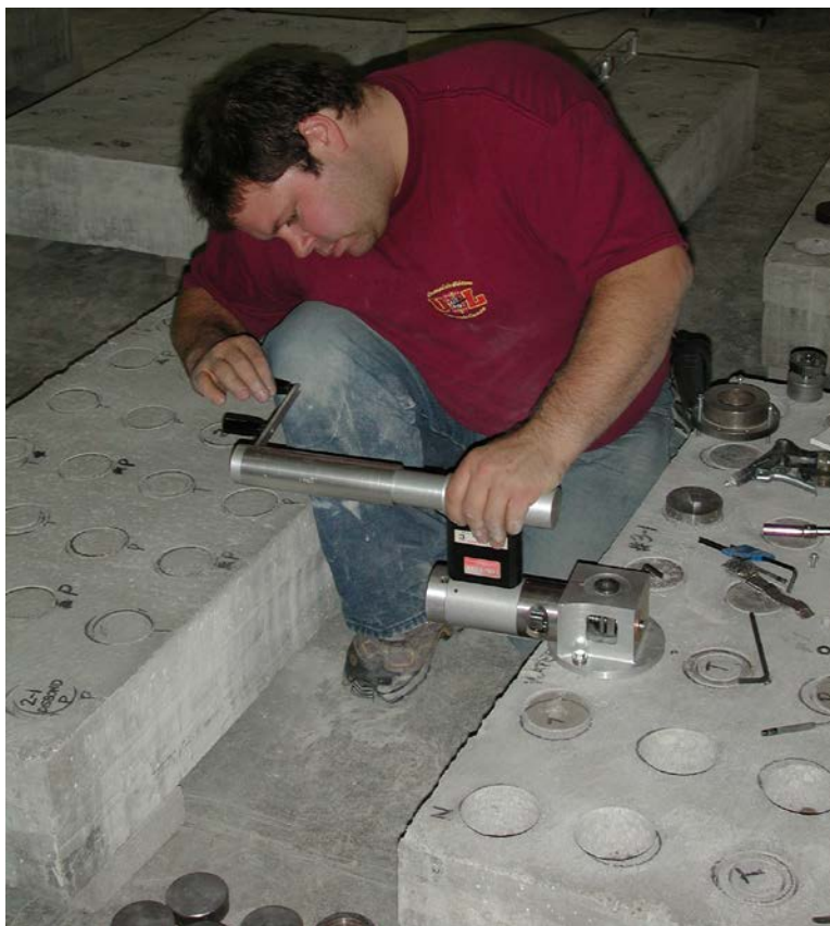
Figure 4. Direct tension bond testing (tensile bond) procedure
