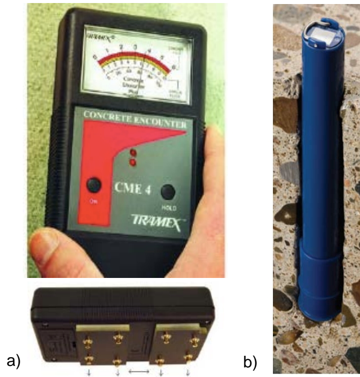
Figure 1. Devices used to monitor the moisture condition in the surface layer of the concrete specimens: a) electrical impedance surface moisture meter; b) embedded relative humidity probes
