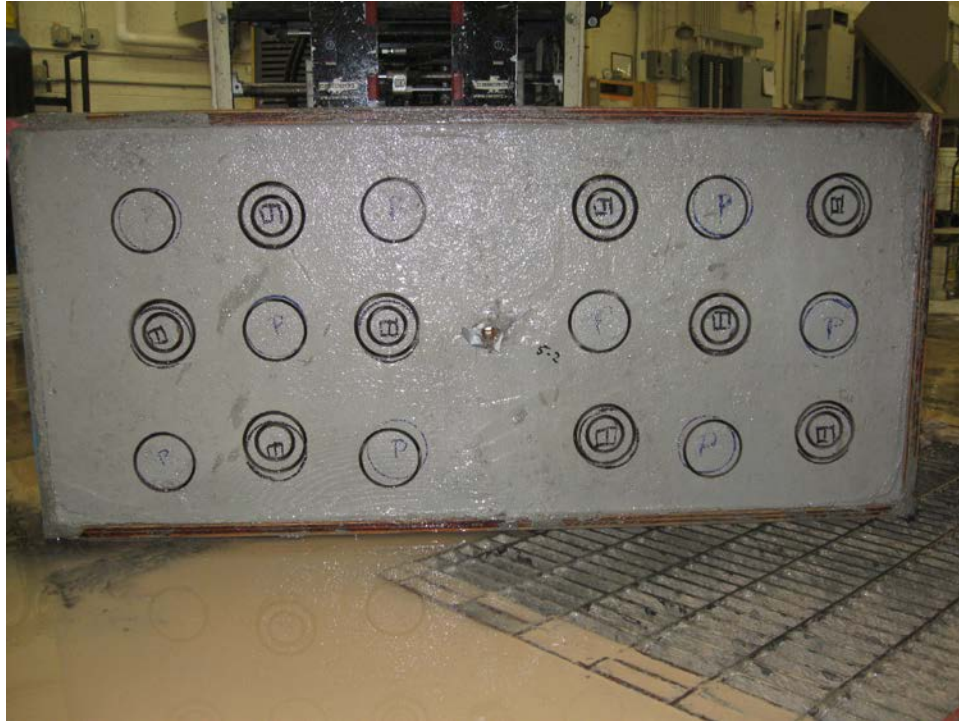
Figure 3. Cored test slab prior to bond testing (single coring: tensile bond; dual coring: shear bond)
