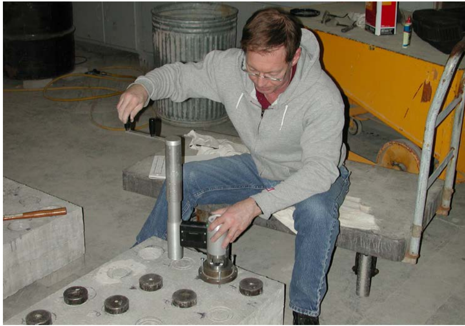
Figure 4. Direct tension bond testing (tensile bond) procedure
