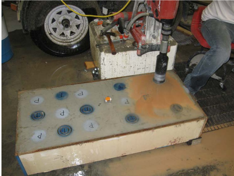
Figure 2. Experimental bond testing preparation (coring template and jig assembly)
