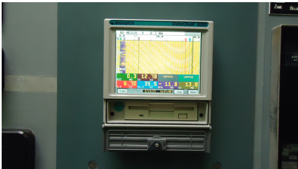
Figure 15 Monarch Data Chart recorder used to log generator power output data.
