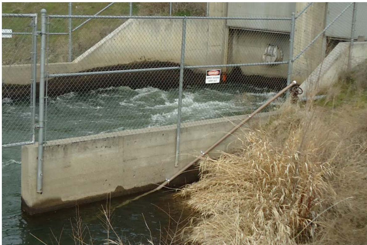
Figure 5 Site #9 Water level logger deployment pipe anchored to the wing wall of the power plant tailbay.
