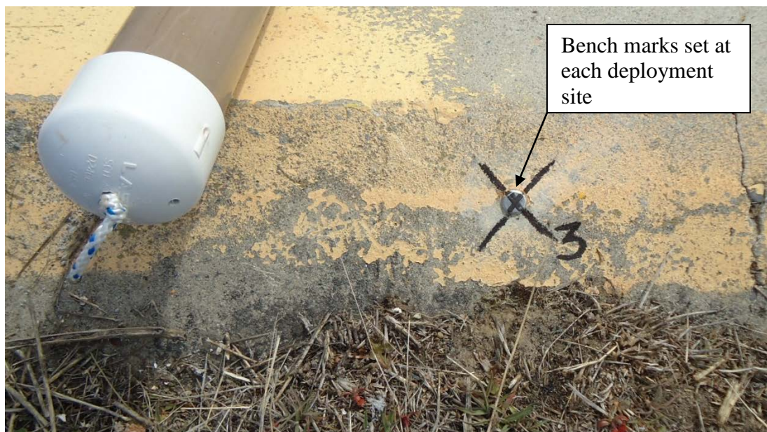
Figure 3 Typical bench mark set at each deployment site marked with a concrete anchor and an X.
