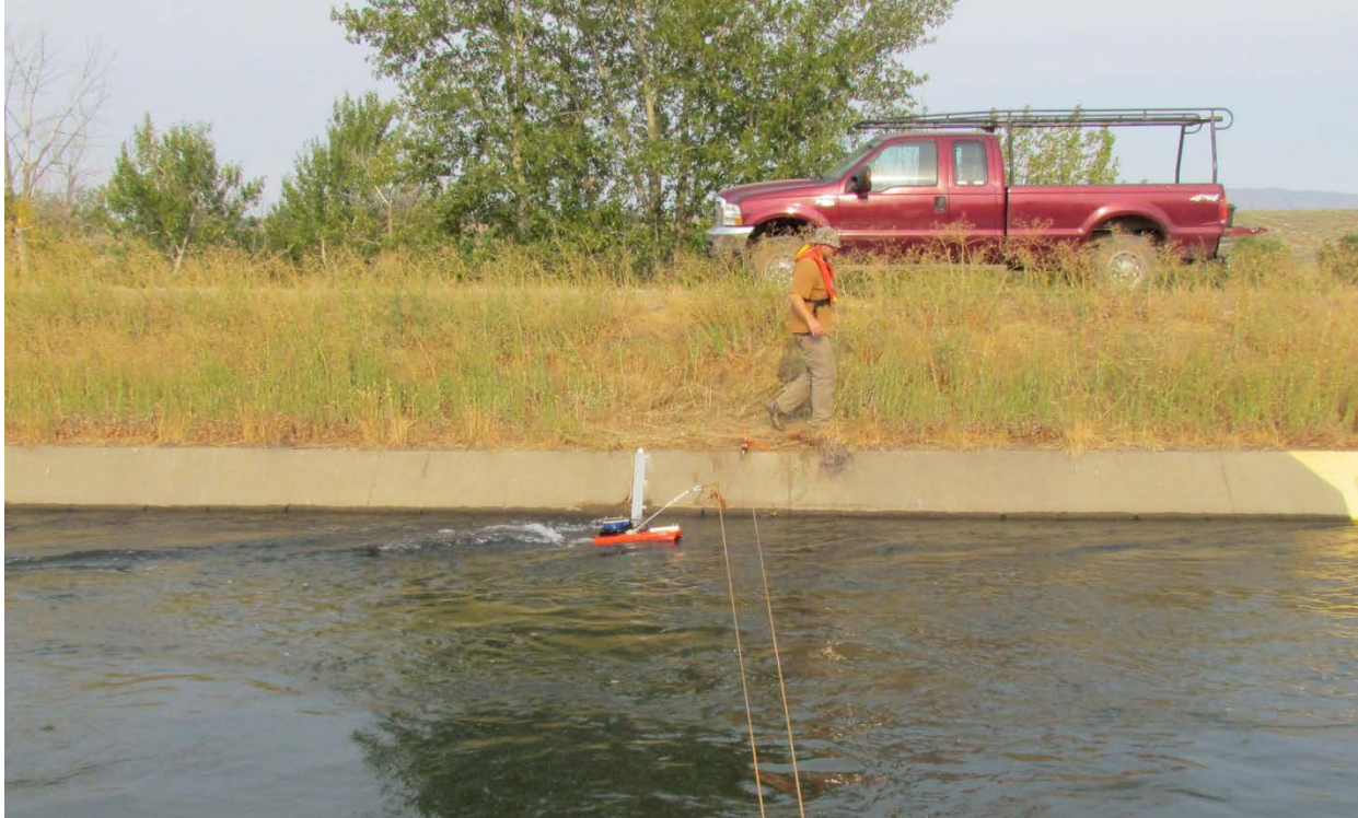
Figure 11 Tagline and StreamPro ADCP at a section upstream of the HK turbine. Canal velocities were measured at the same cross-sections as the water level loggers.
