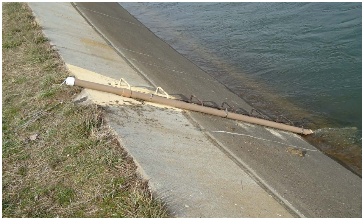
Figure 1 Site #5 water level logger deployment pipe clamped to the downstream side of the safety ladder.
