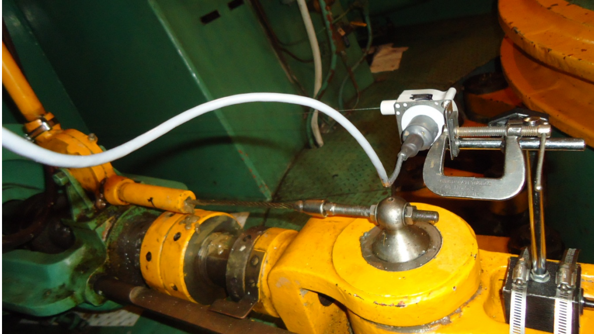
Figure 13 String transducer installed on servo-motor arm to measure wicket gate opening.
