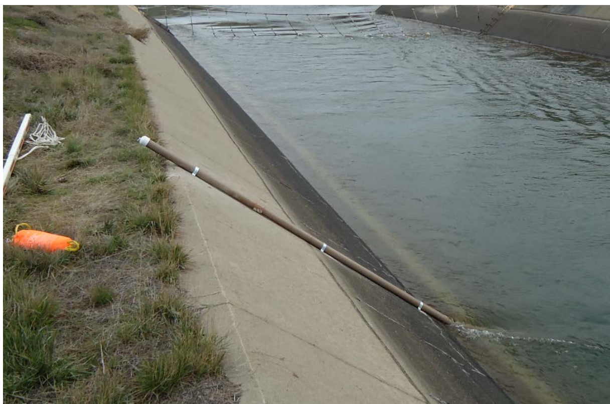
Figure 2 Site #6 water level logger deployment pipe anchored to the concrete side.
