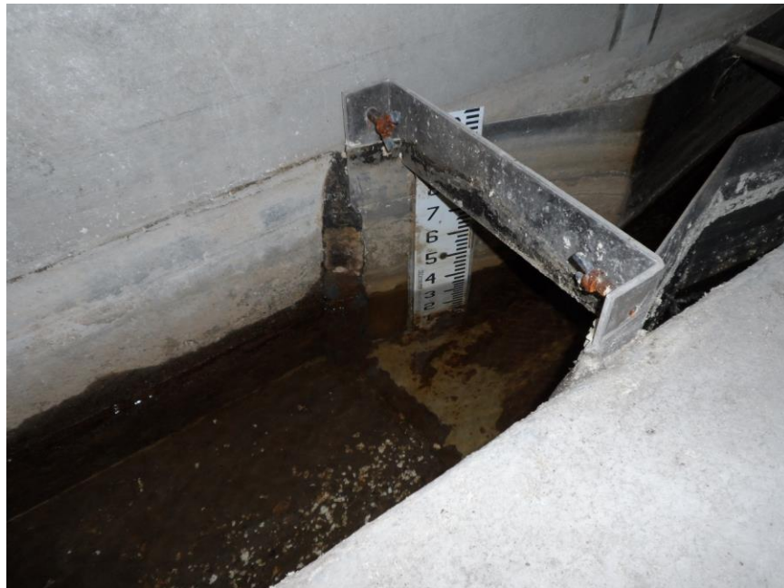
Photo 4.—Weir placed in the 1000 gallery drainage ditch measuring inflow coming from the 81/82 joint area.
