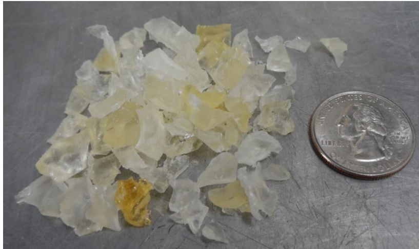
Photo 3.—Ground-up version of Cylutions waterstop.
