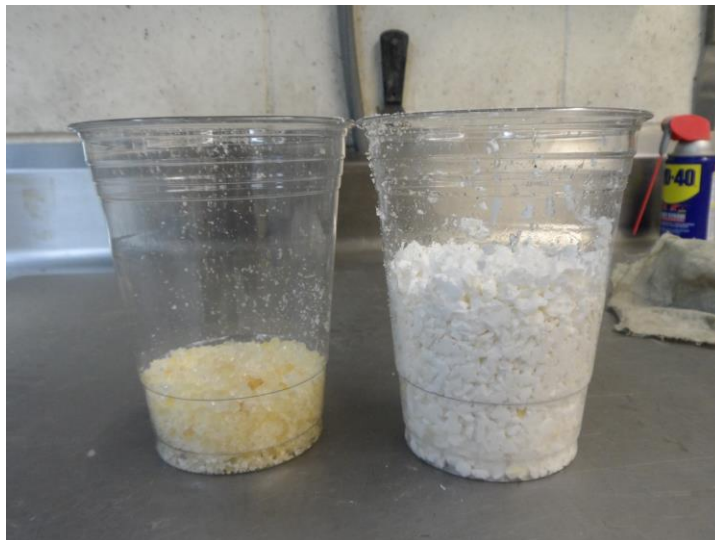
Photo 2.—Ground up waterstop. The left side shows the product before contact with water and the right side right shows the product after water was added. The cups contain the same volume of waterstop material.
