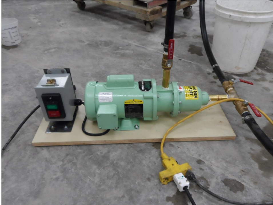
Photo 6.—Progressive cavity screw pump used to deliver water/waterstop solution.
