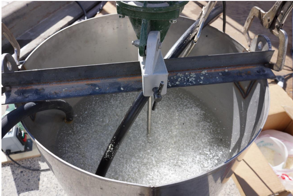
Photo 5.—Ground-up waterstop suspended in water.
