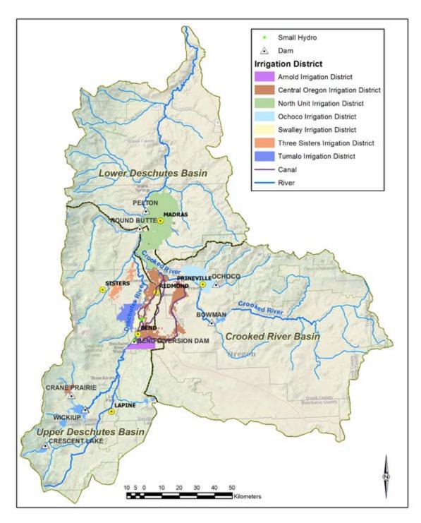
Figure 1: Deschutes River basin showing three major subbasins, existing dams, hydropower facilities, and irrigation districts and canals.
