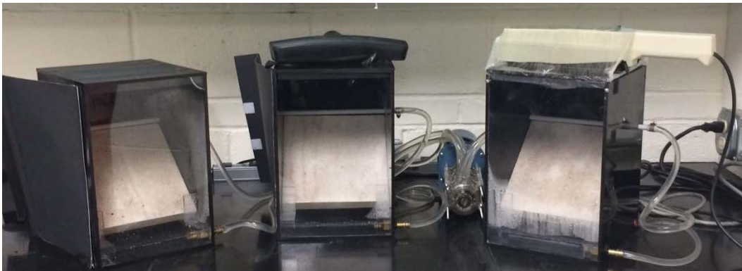
Figure 1. Weathering test experiments running TX Active concrete samples. From L to R: no light, visible light exposure, ultraviolet light exposure.
