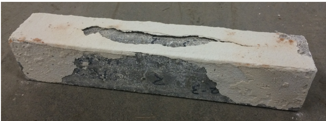
Figure 3. i.active-COAT on an OPC concrete sample after freeze-thaw testing. Note the cracking, delamination, and spalling of the coating.
