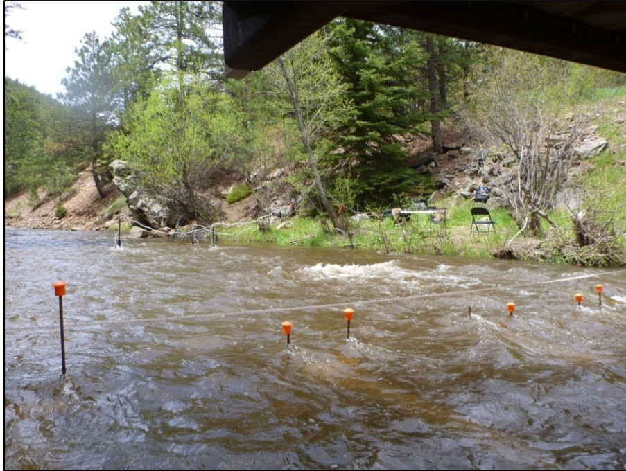
Figure 4: Photograph (looking upstream) of bed load traps (foreground) and hydrophones (background) deployed on Bear Creek near Evergreen, CO.
