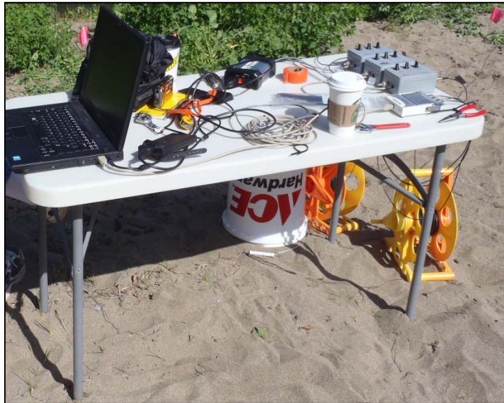
Figure 3: Photograph of the first iteration of the passive acoustic bed load monitoring system, deployed at Douglas City on the Trinity River, CA
