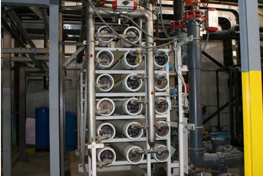
Reverse osmosis process (NGL Water Solutions, used by permission).
