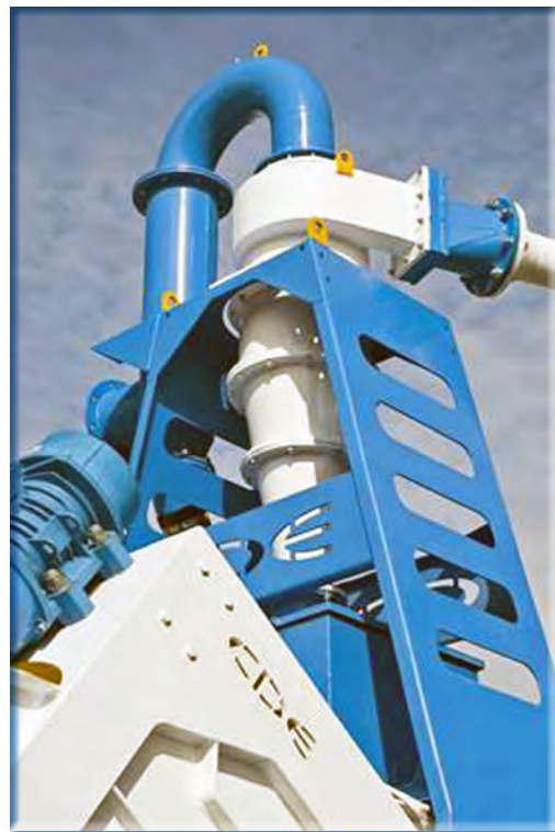
Hydrocyclone Separator (CDE Global Inc., used by permission).
