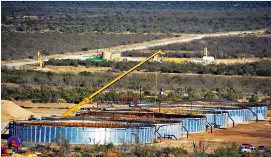
Apache uses above ground modified grain bins with double-layer plastic liners to hold and treat produced water that is recycled for use in Wolfcamp shale wells in Irion County, Texas (Apache Corp., used by permission).
