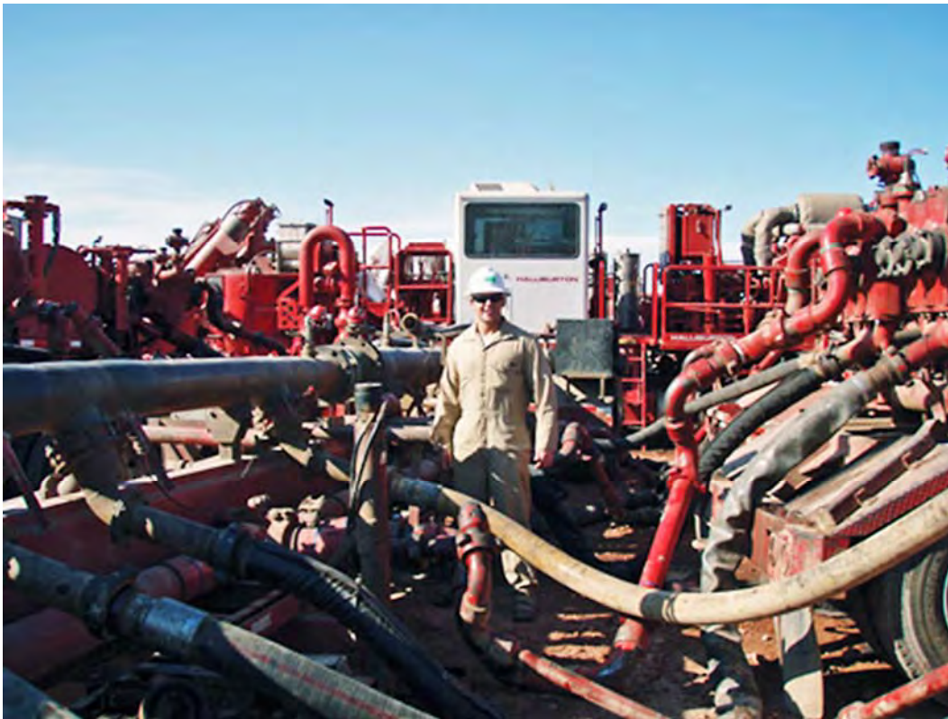
Process of mixing water with fracking fluids to be injected into the ground (Wikimedia commons).
