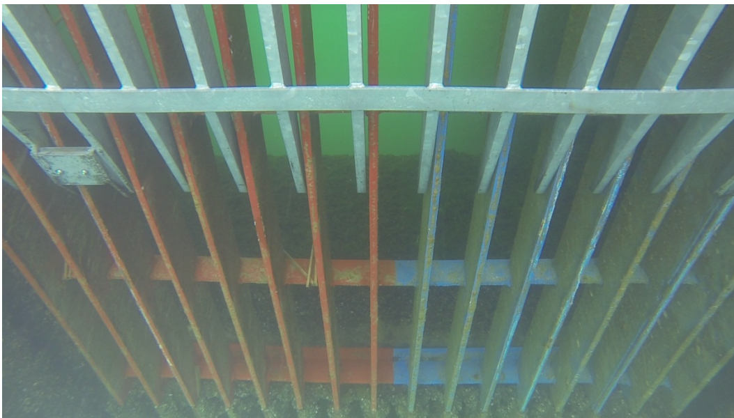
Figure 9.—Video still captured from May 2014 inspection—red PPG Sigmaglide 890 (left), blue Seacoat Seaspeed V5 (right).
