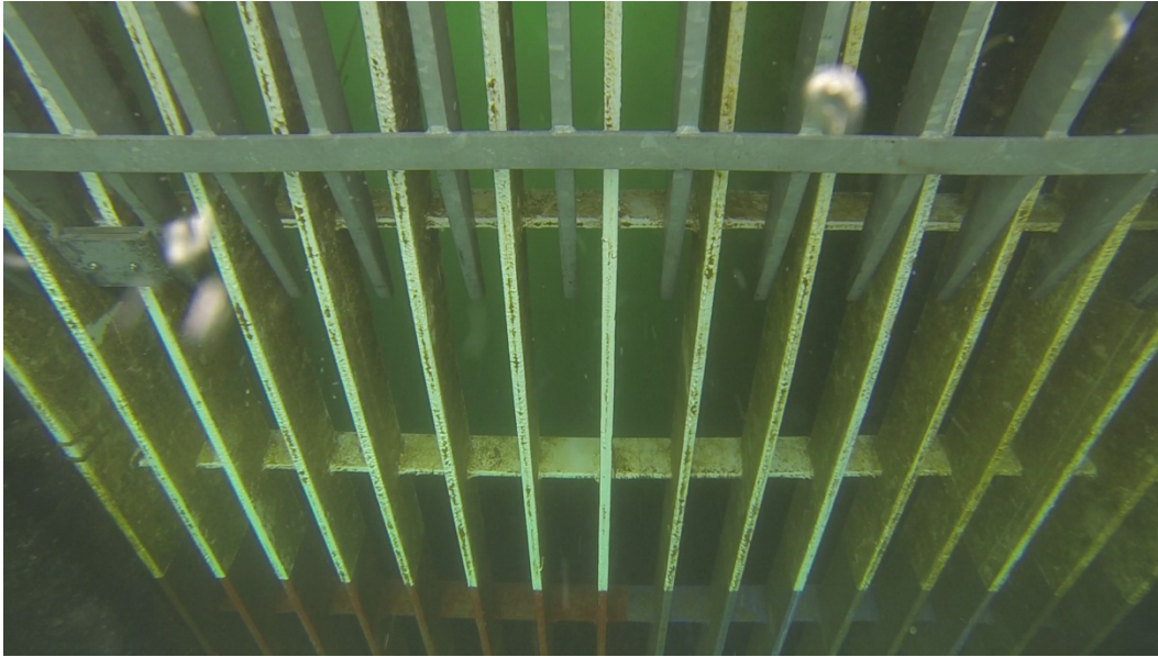
Figure 8.—Video still captured from May 2014 inspection—white International Intersleek 970 (left), white Fuji Sher-Release (right).
