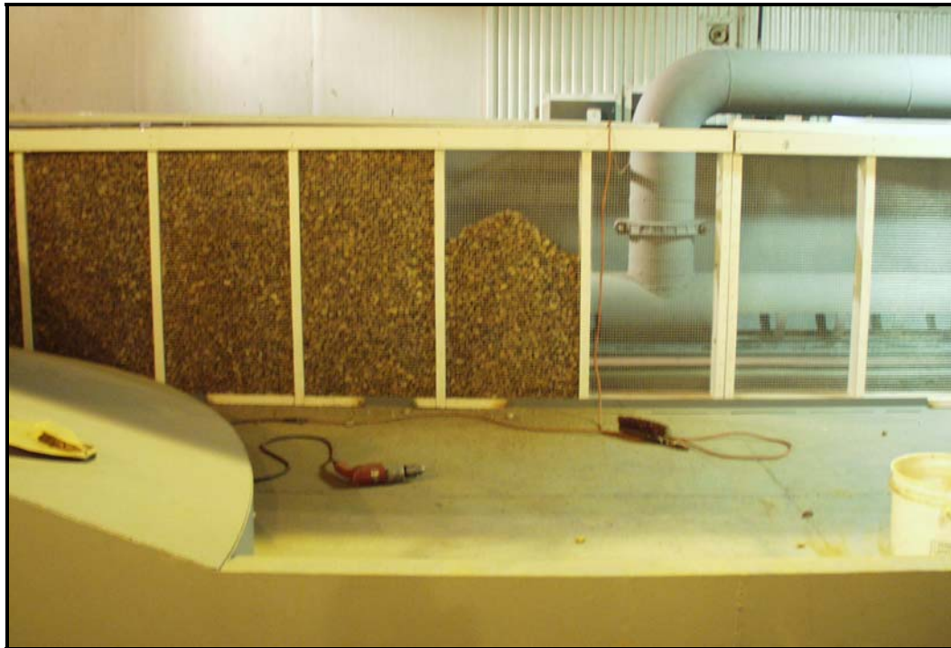
Figure 3.5: Headbox Under Construction Including Pipe Manifold and Rock Baffle (Figure 3.5 in Heintz (2002))
