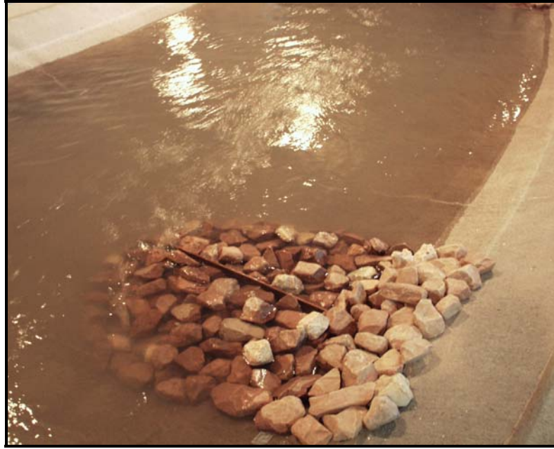
Figure 3.19: Impermeable Bendway Weir during Testing
