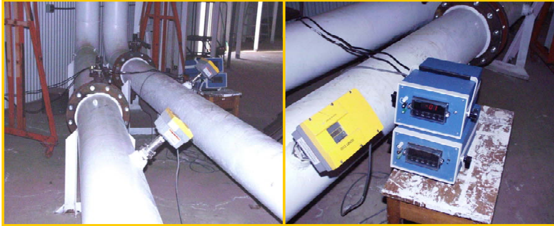
Figure 3.3: SIGNET 2550 Insertion Magmeters and Digital Display Boxes (Kinzli 2005)
