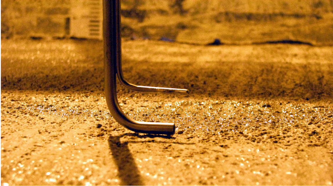
Figure 3.9: Preston tube on the surface of the concrete cap in the 4-foot flume.
