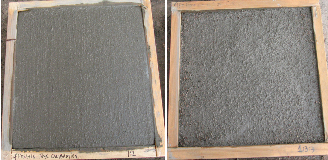
Figure 3.7: Two tests of concrete mixture for the concrete cap: Cement:Sand ratio of 1:2 (left) and Cement:Sand:Gravel ratio of 1:3:3 (right).
