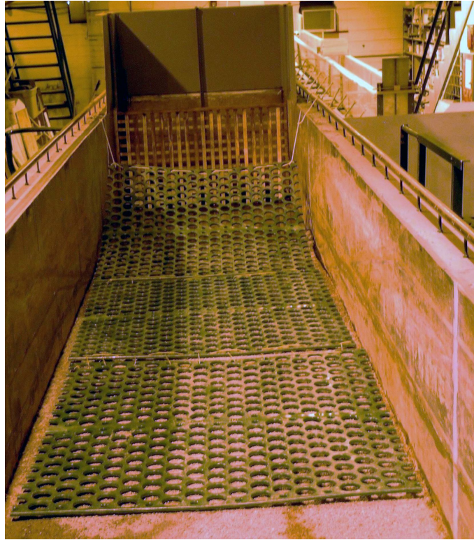
Figure 3.12: Scour stop mats installed at the upstream end of the 4-foot flume.
