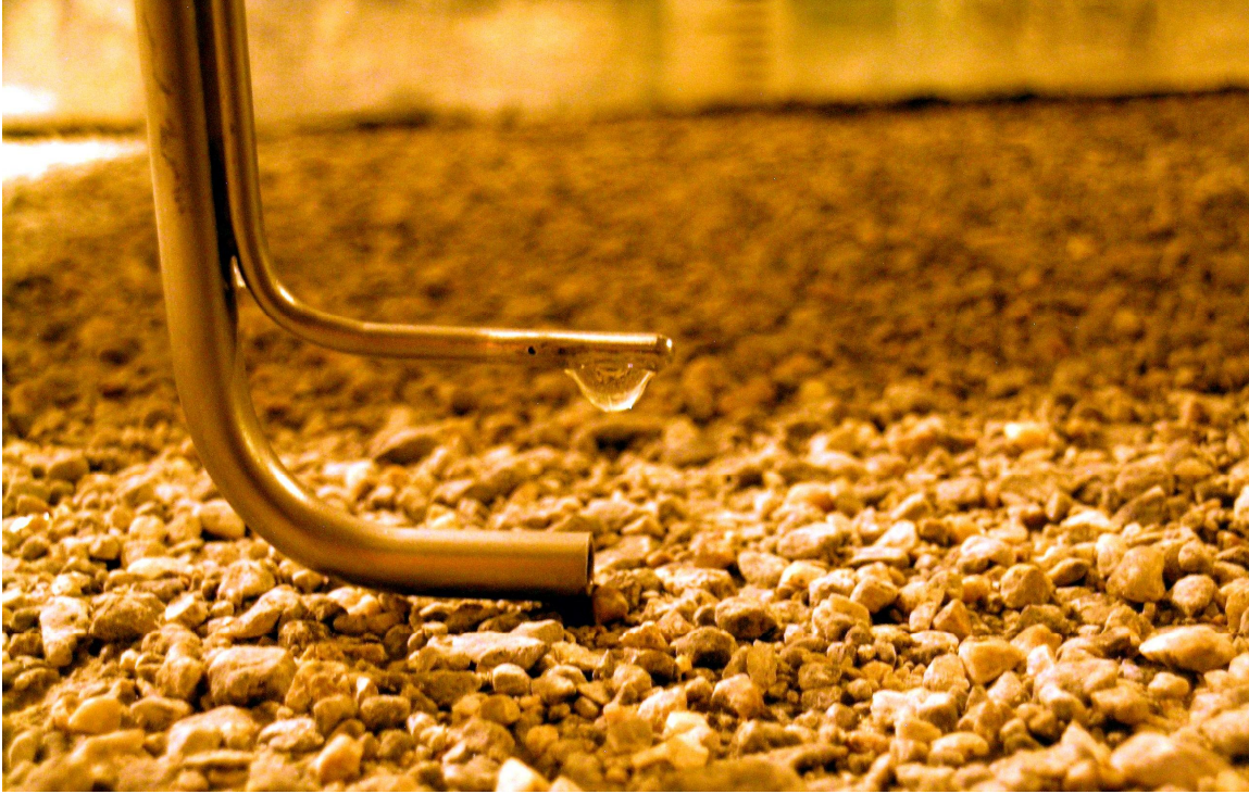
Figure 3.4: Preston tube on the surface of the gravel bed in the 4-foot flume.
