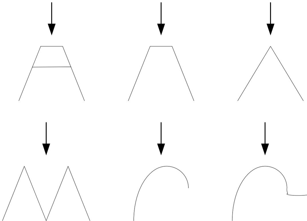
**Figure 2. Depiction of Weir Structure Types. Arrows indicate direction of flow.**
