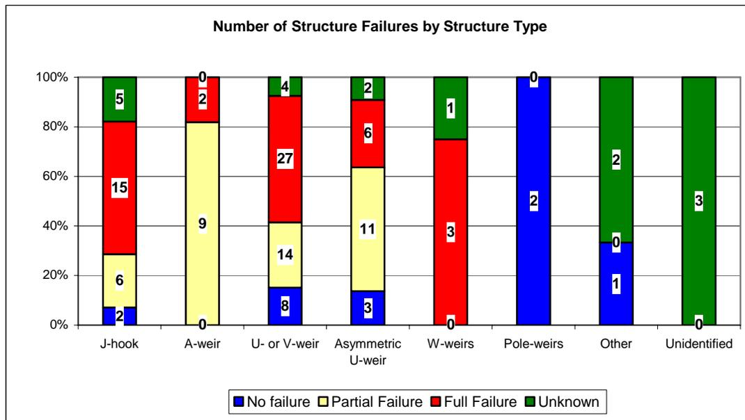
Figure 14. Number and Percentage of partial and full failures for each type of structure.
