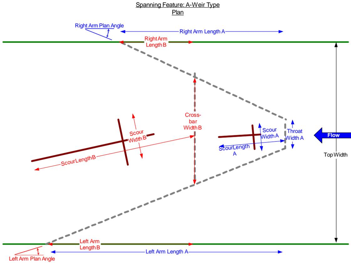
**Figure 1. Example Component Diagram using an A-Weir Structure**
