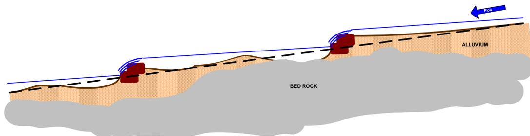
Figure 17. Longitudinal Profile of Sediment Deposition and Pool Patterns
