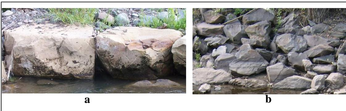
**Figure 8. Rock Shape a) Blocky versus b) Angular**
