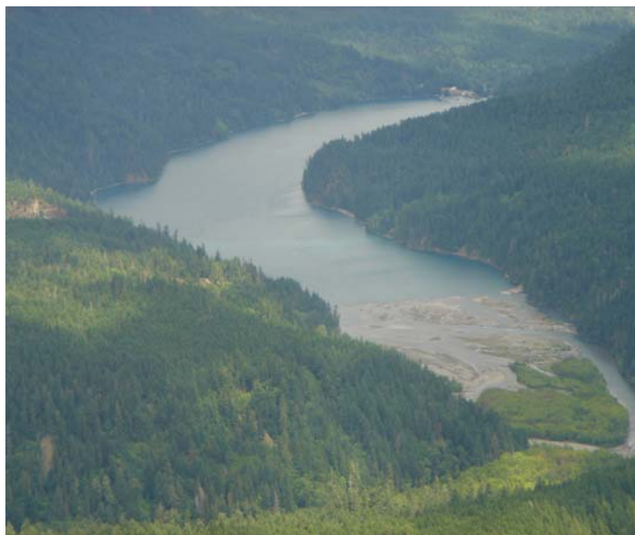
Figure 3. Photograph looking downstream at Lake Mills, behind Glines Canyon Dam, and the reservoir delta composed of sand, gravel, and large woody debris.
