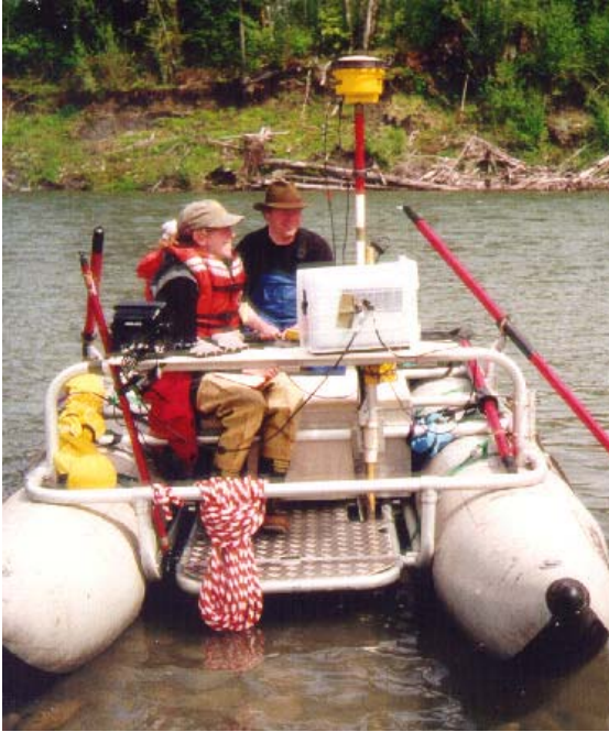
Figure 20. View of survey boat configuration equipped with global positioning software (GPS) equipment, depth sounder, and laptop to document channel bathymetry.
