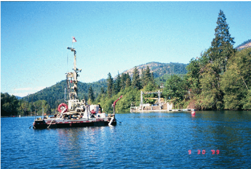
Figure 19. View downstream showing Reclamation's custom built, floating drilling platform in operation on drill hole AP-99-10. The spillway and pumping plant portions of Savage Rapids Dam are present in the background of this photograph. (Reclamation photograph by Richard Link; September 30, 1999.)
