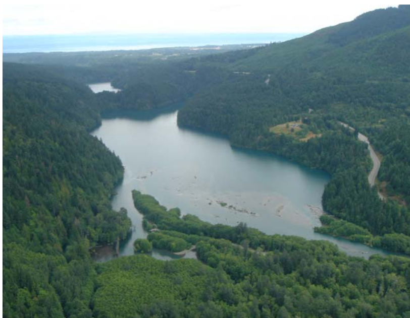
Figure 4. Photograph looking downstream at Lake Aldwell, behind Elwha Dam, and the reservoir delta composed of sand, gravel, and large woody debris.
