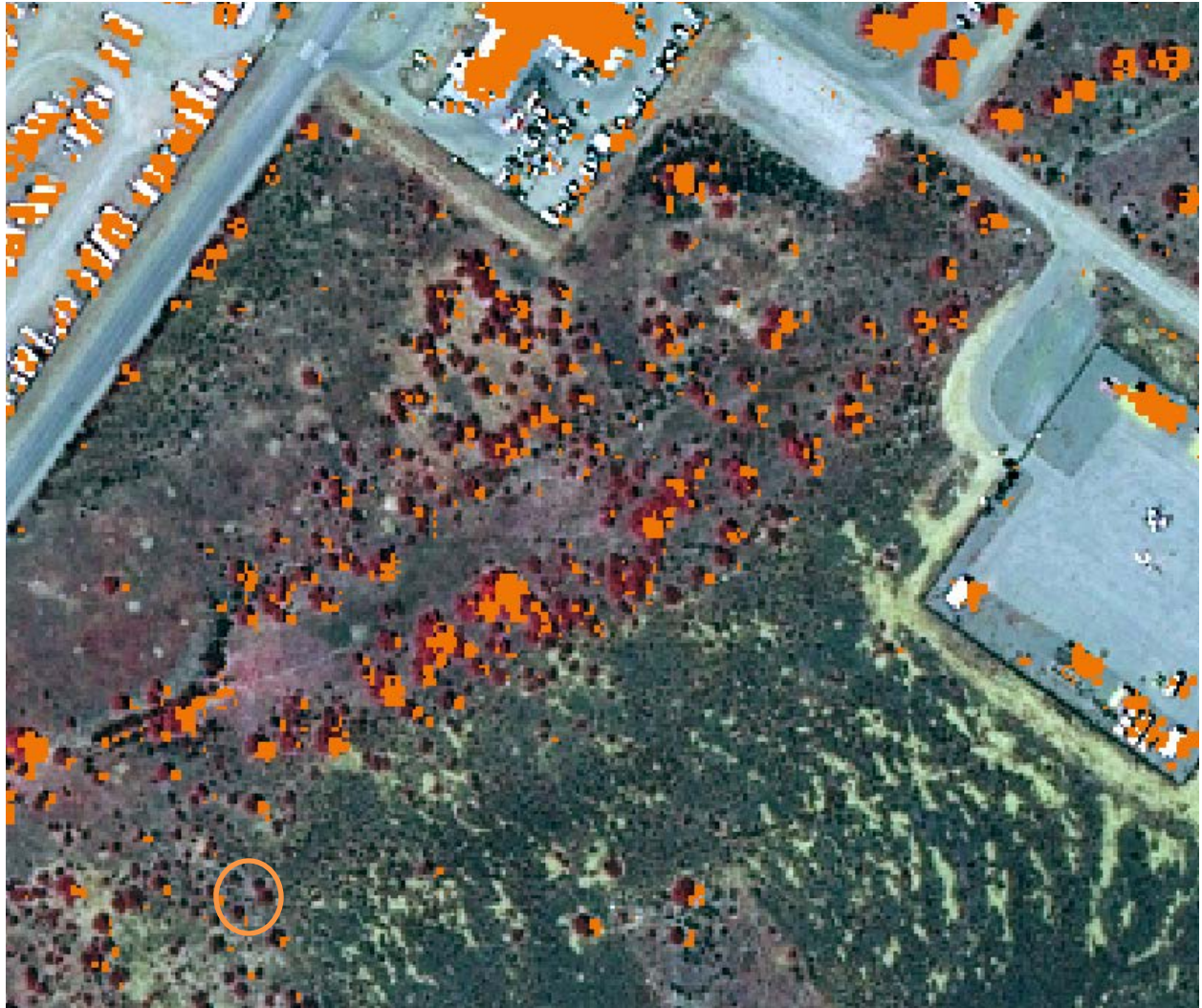
Figure 8: Pixels with height above the ground are displayed in orange. This image shows areas of misregistration along with shrubs that were not captured by the LiDAR data at all (small orange circle at bottom left hand corner).
