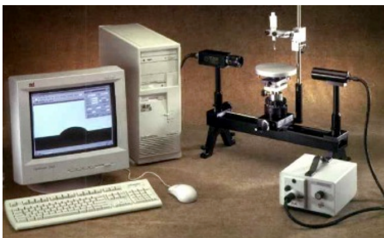
Figure 5.—Goniometer apparatus used for contact angle measurements.
