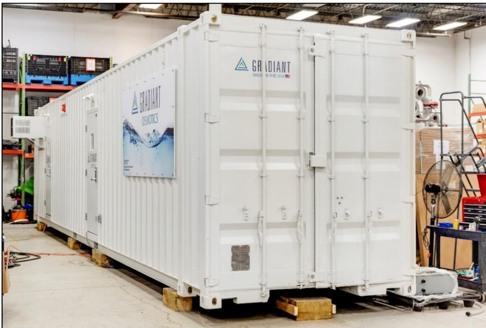
Figure 3. CFRO pilot unit in the fabrication shop.
