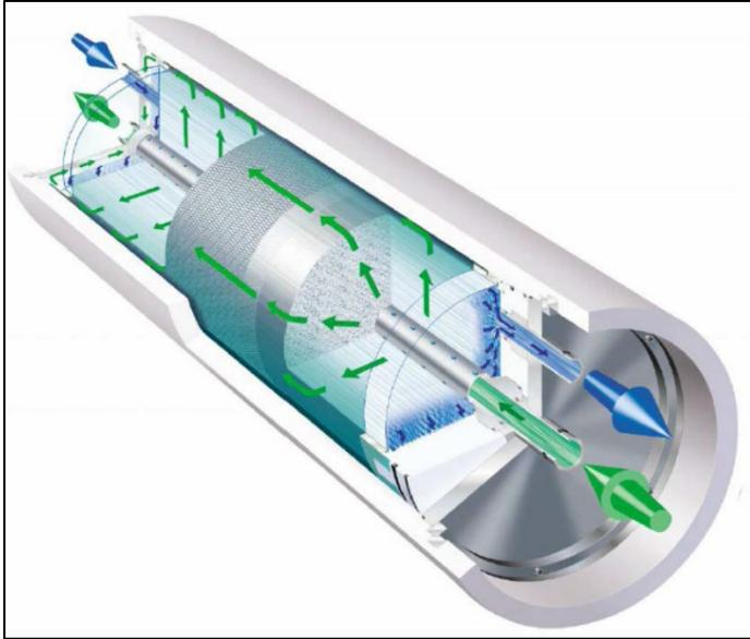
Figure 2. Flow pattern in the CFRO membrane
