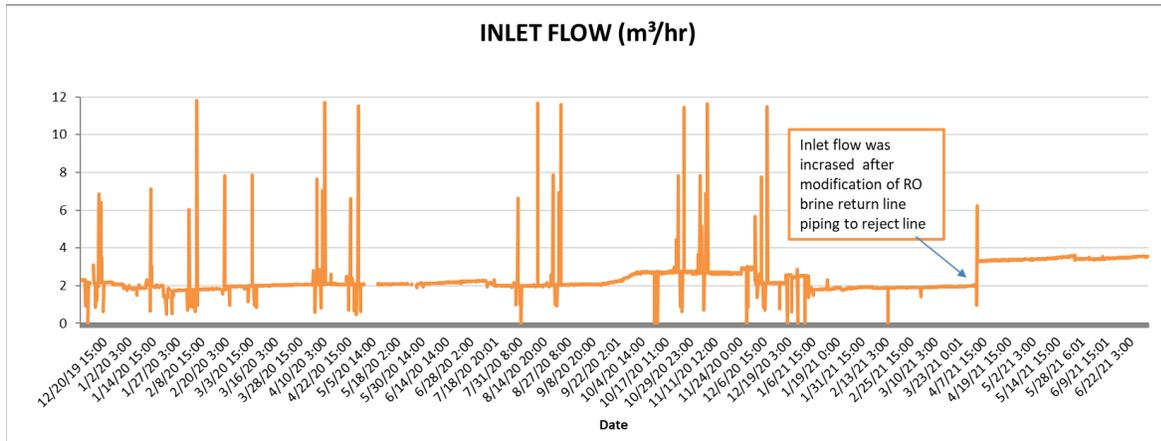
Figure 10. Inlet flow rate
