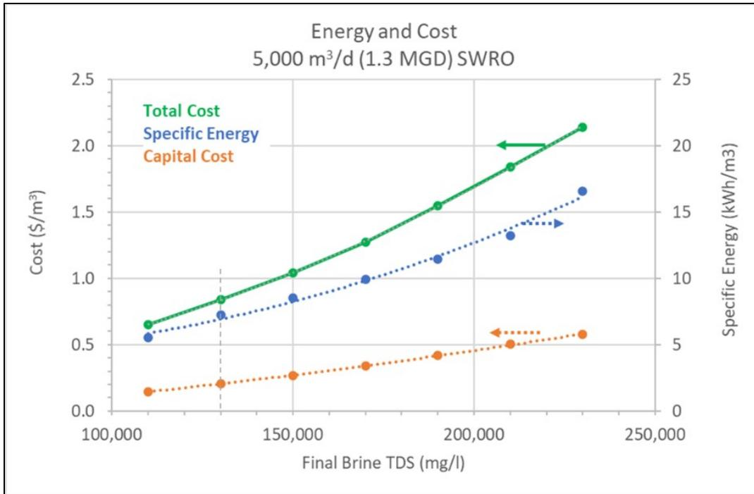
Figure 20. Projected costs and energy requirements for a full-scale CFRO plant
