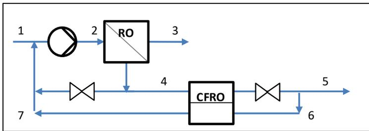
Figure 1. CFRO pilot unit process flow diagram
