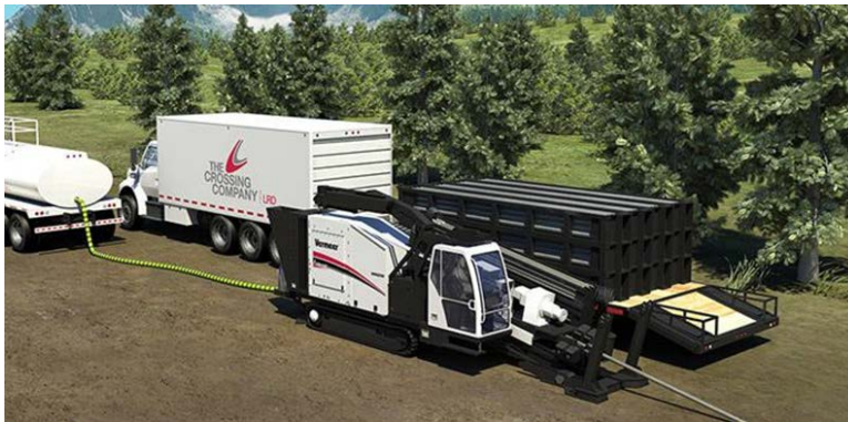
Figure 4. Typical HDD Light Rig Setup (The HDD Co.)
