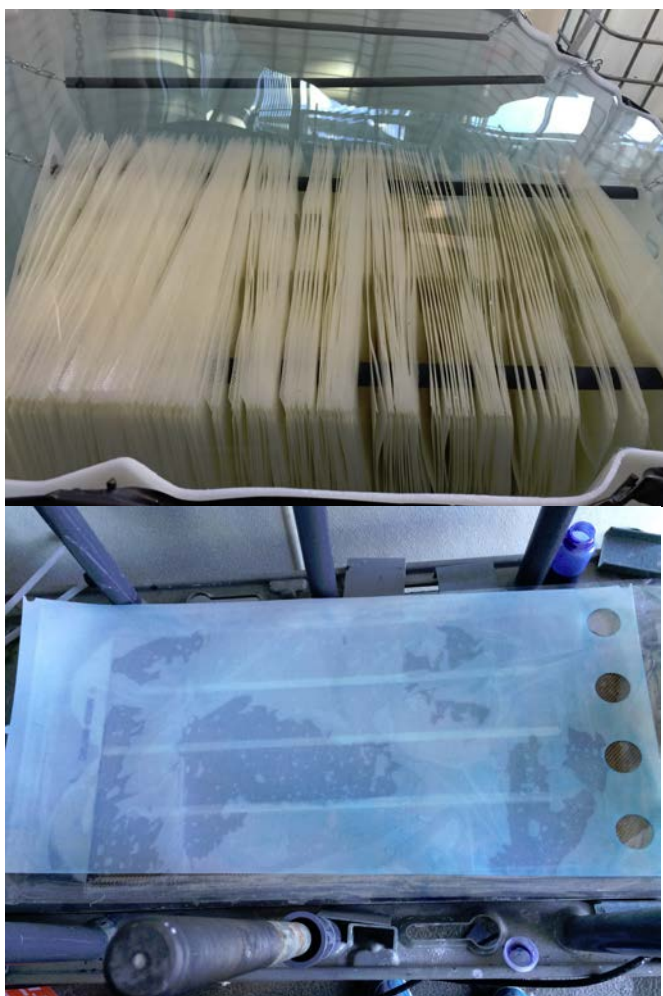
Figure 6.—Coating cation selective membranes CR671 and coated membrane passed dye testing.
