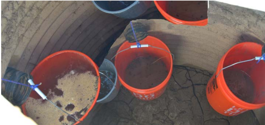
Figure 16. Culvert drain buckets following a flood event. Note full to near empty buckets.
