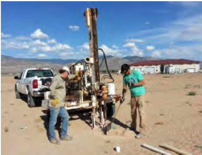
Figure 4.—UA drilling port access holes for monthly neutron probe measurements.
