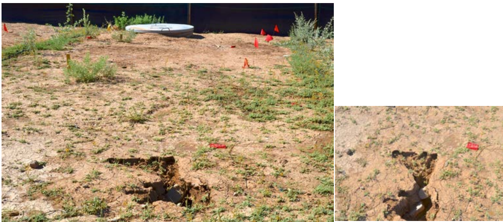
Figure 17. Soil surface failure showing deep channeling following a flood event.
