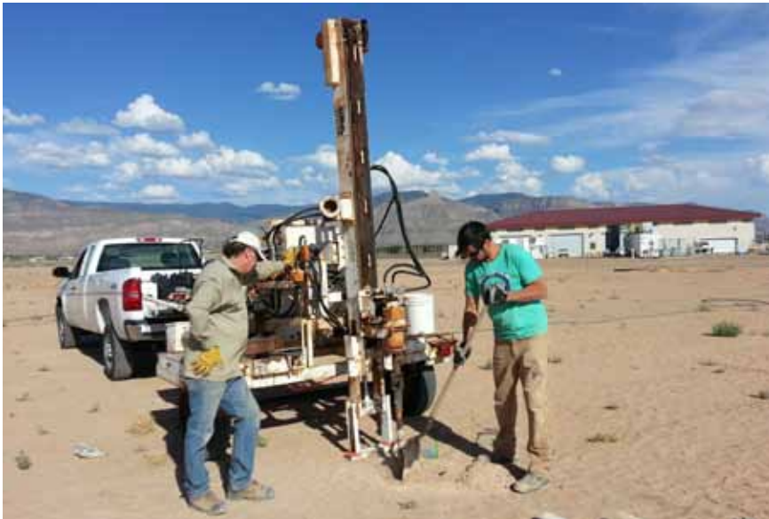
Bob Seaman, Research Technician (left) and Ryan Furcini, graduate student (right), University of Arizona, drilling data port holes for neutron hydroprobe readings
