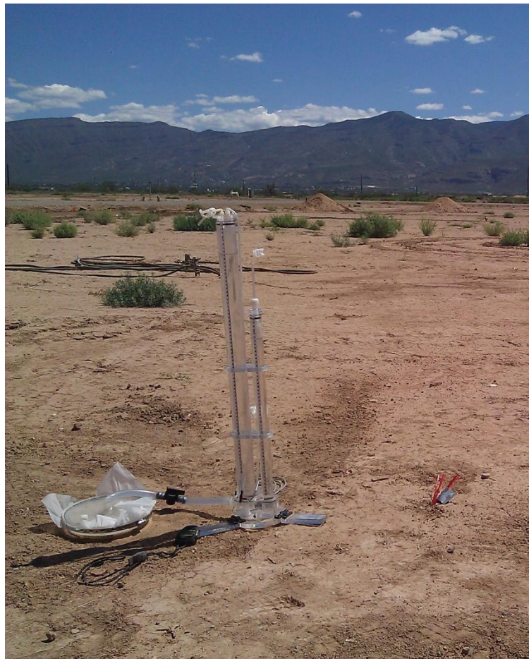
Fig. 1. Infiltrometer installed for infiltration tests at the Brackish Groundwater National Desalination Research Facility, Alamogordo, NM on August 28, 2014
