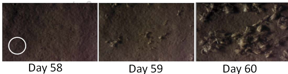
Figure 26. MMS images at days 58-60, indicating mineral scale detection (detection point 2 in Figure 22), within three days after the SIMS recovery was raised to 68% (at day 57). Initial antiscalant dose: 5 ppm AS1. Antiscalant dose was raised to 6-7 ppm in day 59-60. RO average flux: 13 GFD, feed salinity ~9,000 mg/L TDS.
