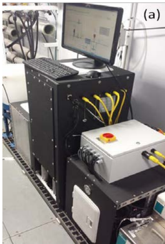
Figure 11. UCLA Membrane Monitoring System (MMS) deployed in the UCLA SIMS. The MMS can be connected to various streams (e.g., UF feed and filtrate, RO feed and concentrate) from the UCLA SIMS.
