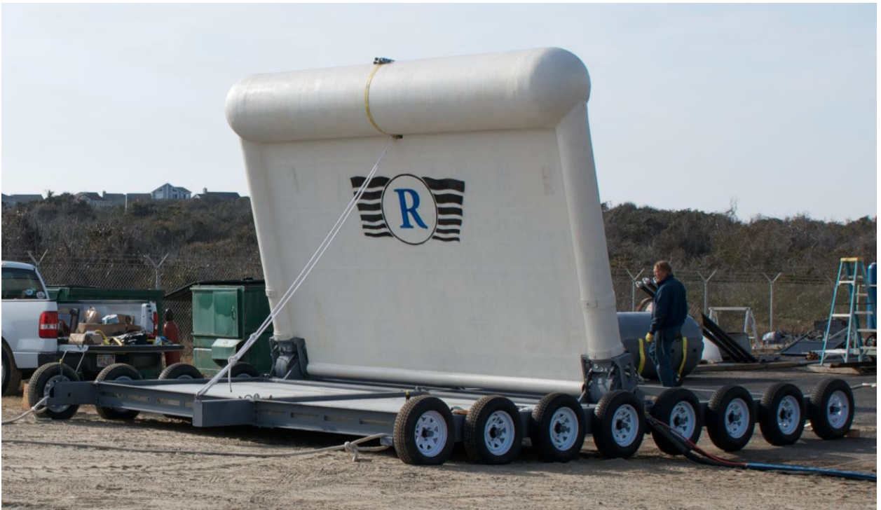
Figure 29. Fully Assembled SurgeWEC and PTO Subassembly
