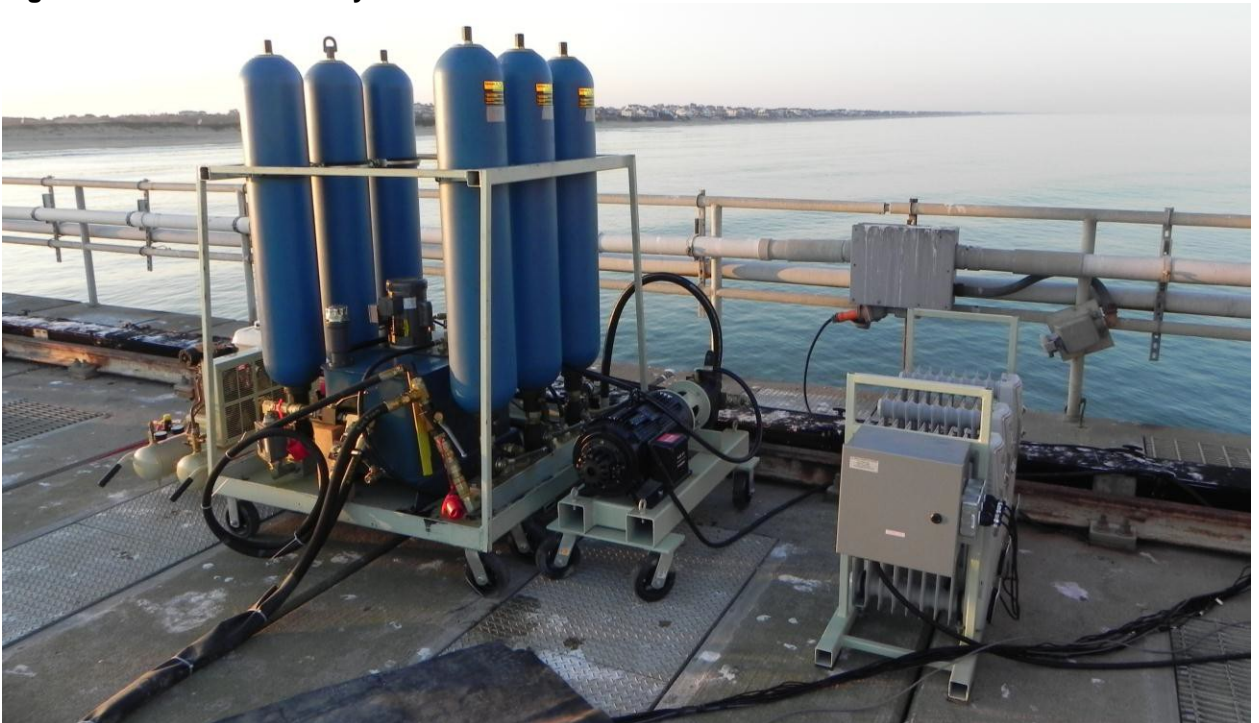
Figure 27. Pressure/Flow Regulation, Generator, and Load Bank Subassemblies
