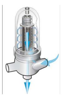
Figure 2-14 Spin Klin Arkal Filter in Normal Filtration Mode
