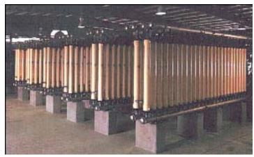
Figure 2-10 Pressure Vessel Configuration Membrane Filtration (Pall Corporation System)
