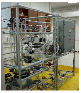
Figure 2-4 Yale University Prototype of Forward Osmosis System
